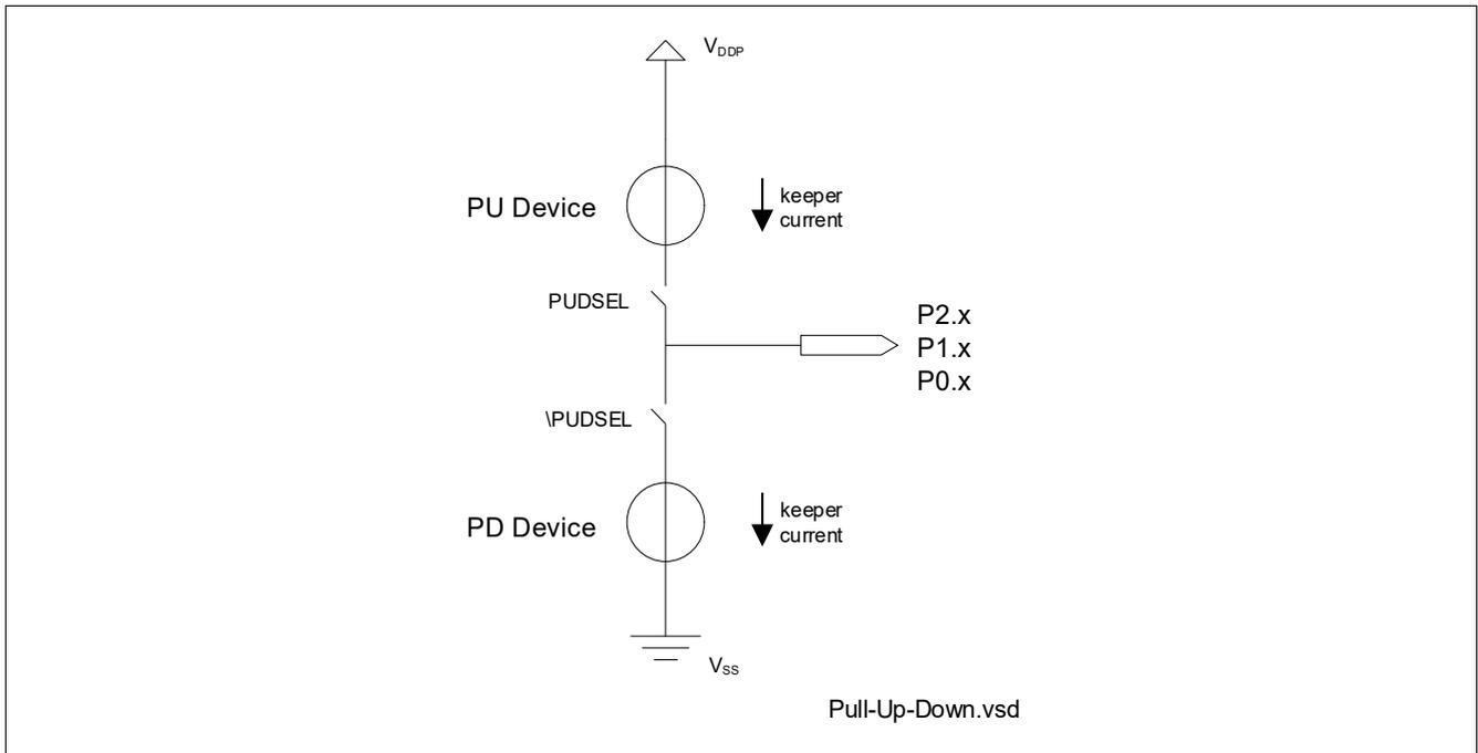
Figure 22 Pull-up/pull-down device
