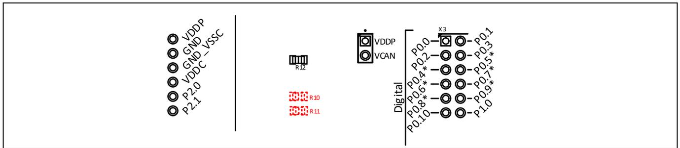
Figure 21 Placement option for R10 and R11
