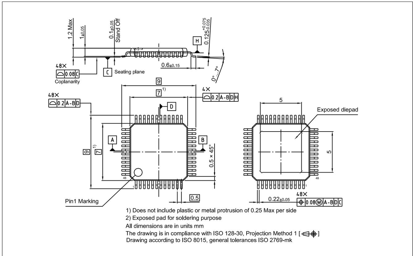
Figure 46 PG-TQFP-48-10
