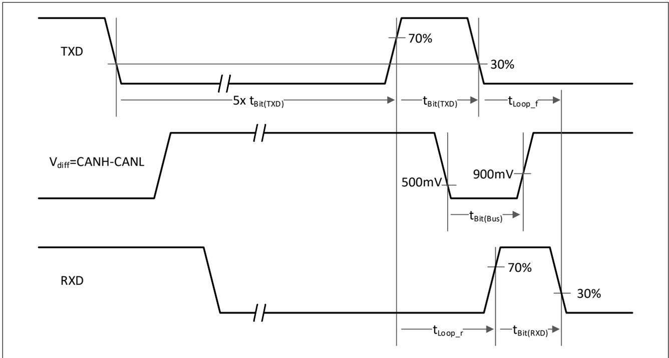
Figure 19 From ISO 11898-2:  $t_{loop}$ ,  $t_{bit(TXD)}$ ,  $t_{bit(Bus)}$ ,  $t_{bit(RXD)}$  definitions
