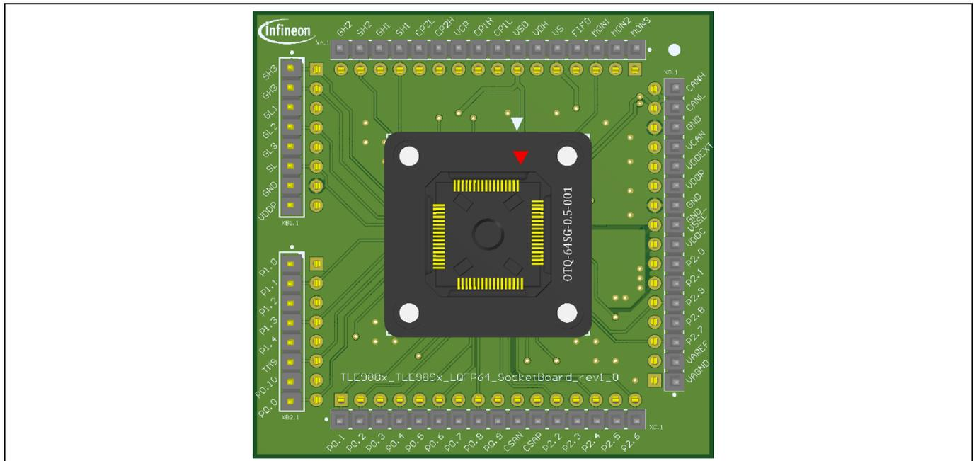
Figure 8 TLE988x\_TLE989x LQFP64 Socketboard (top view)
