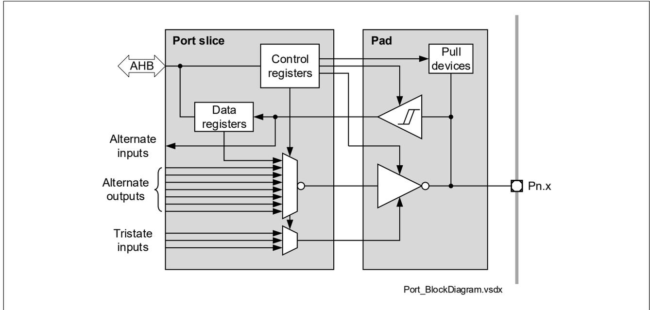
Figure 20 General structure of bidirectional port
