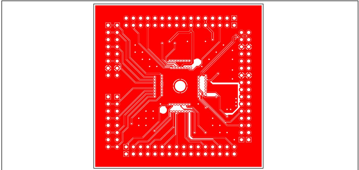
Figure 37 TLE988x\_TLE989x LQFP64 Socketboard, Top layer
