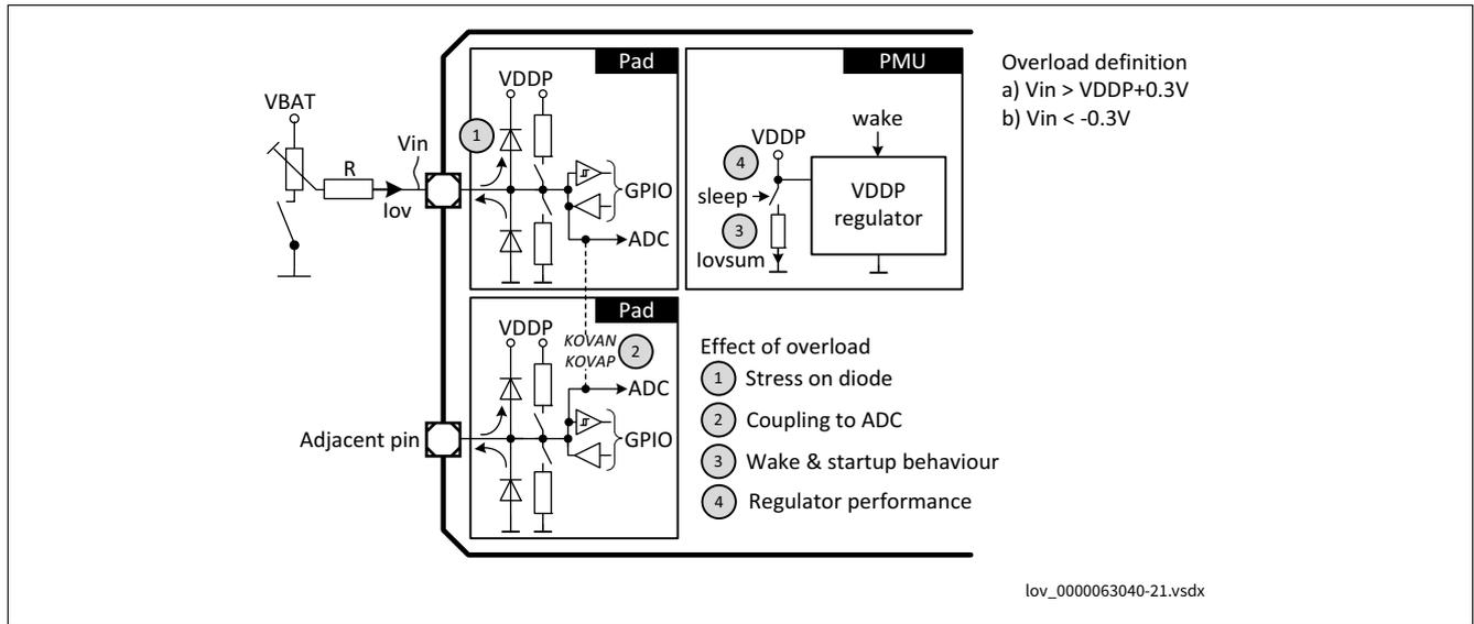
Figure 7 Overload current
