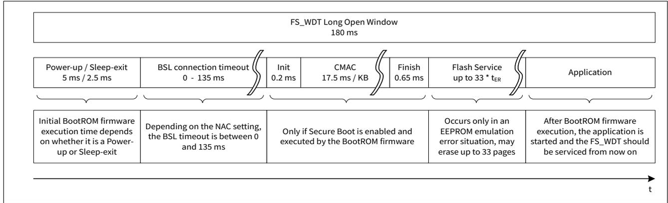
**Figure 5 Device bootup timing**
