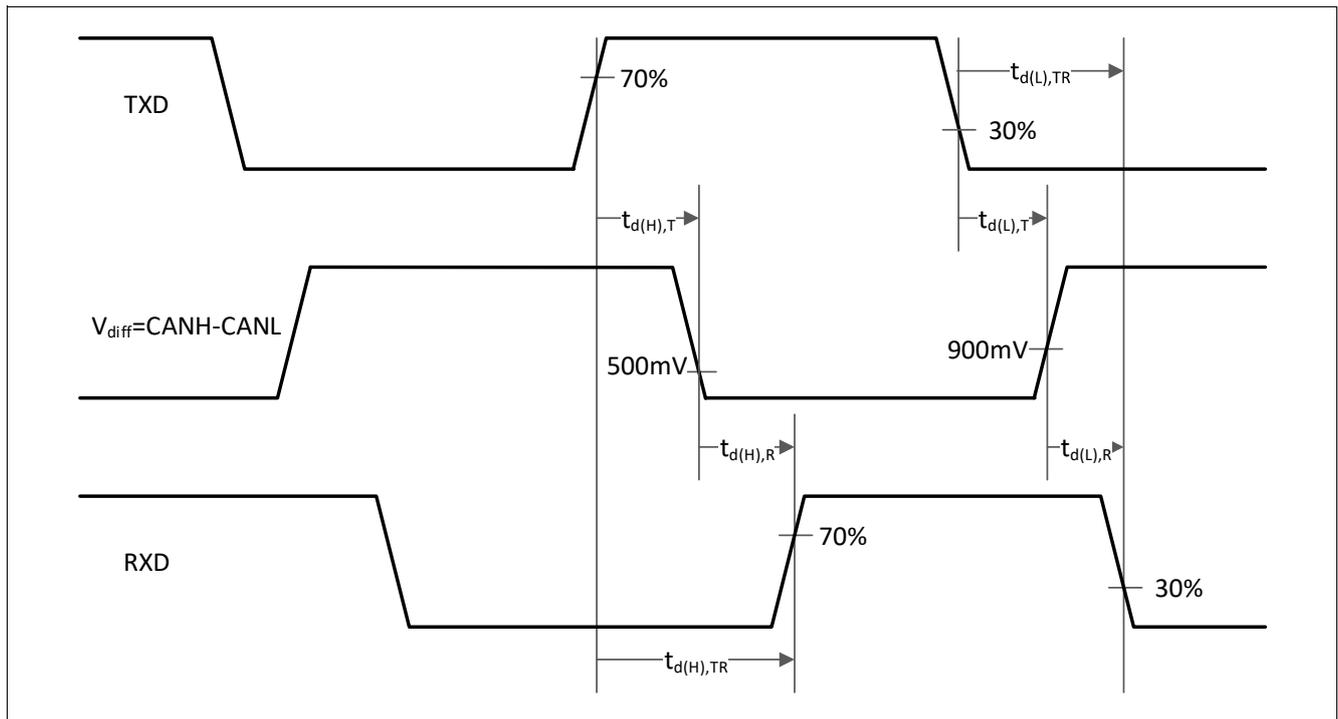
**Figure 18 Timing diagrams for dynamic characteristics**
