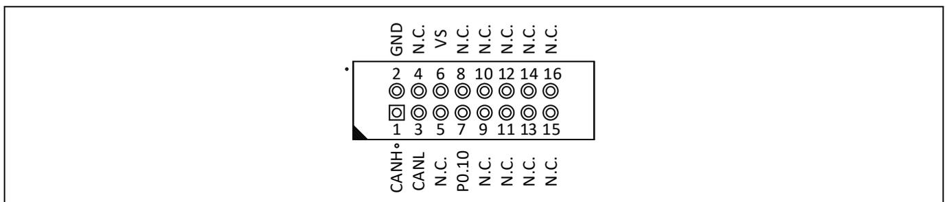
Figure 13 Pinout of CAN\_BSL interface
