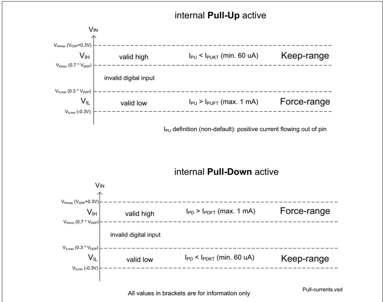
Figure 23 Pull currents, Keep and Force Current
