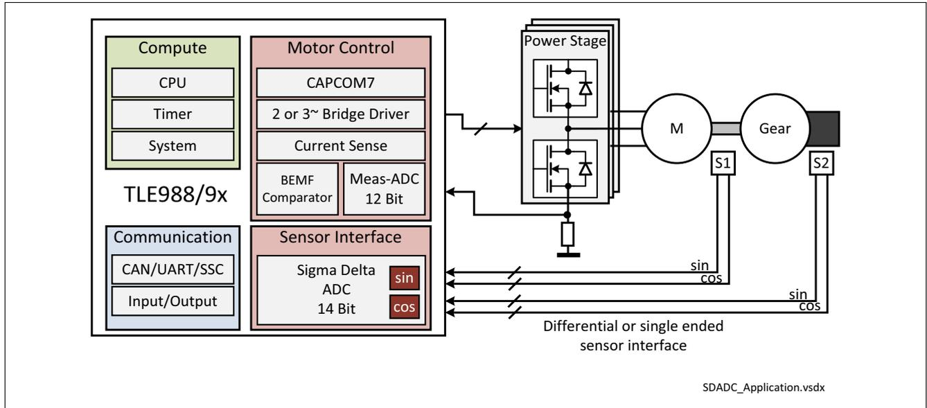
Figure 35 Application diagram SDADC
