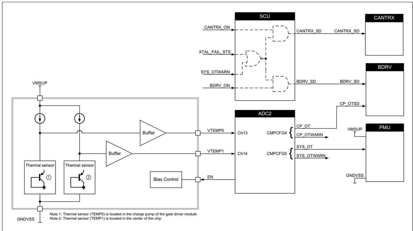
Figure 32 Block diagram TMPSNS
