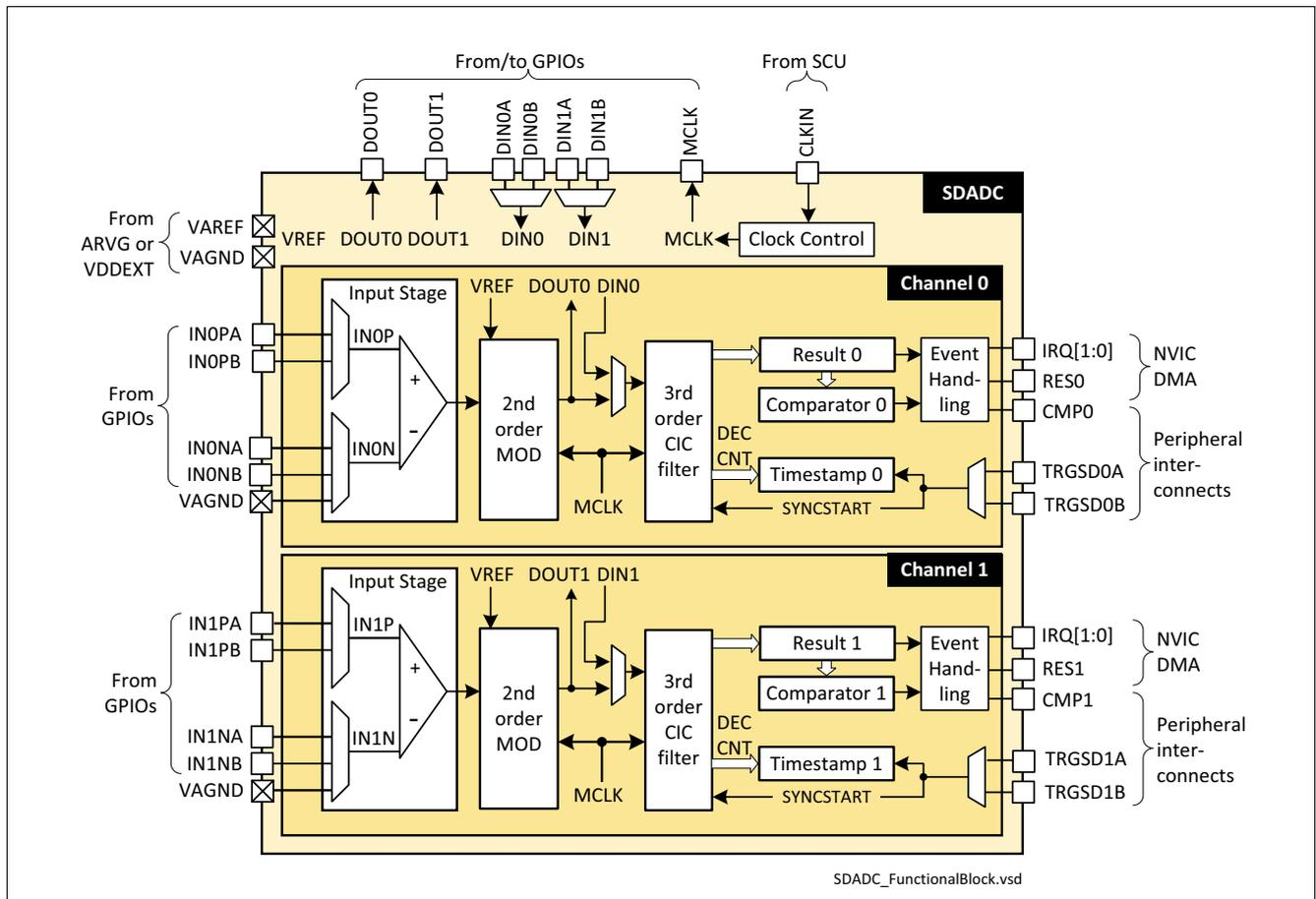
Figure 36 Block diagram SDADC
