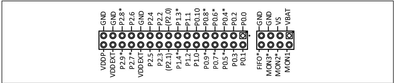
Figure 20 Pinout of X2 (left) and X3 (right)
