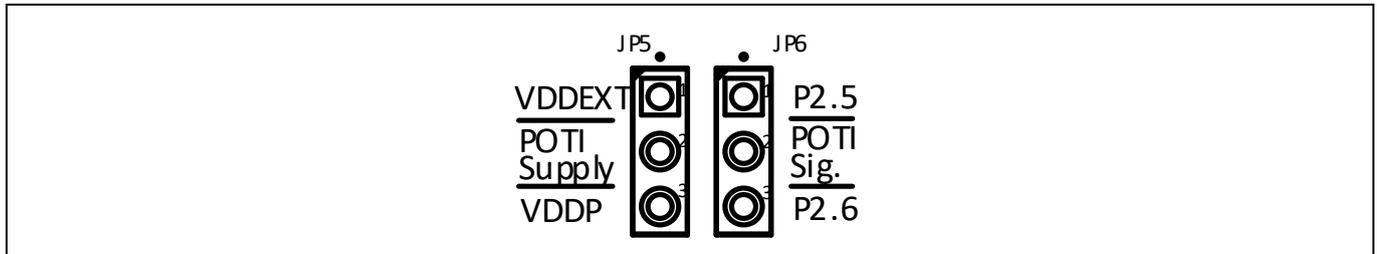
Figure 18 Pinout of JP5 (left) and JP6 (right)
