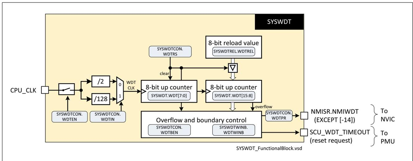
Figure 12 Block diagram SYSWDT
