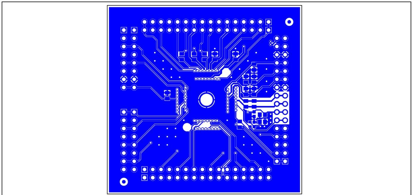
Figure 38 TLE988x\_TLE989x LQFP64 Socketboard, Bottom layer
