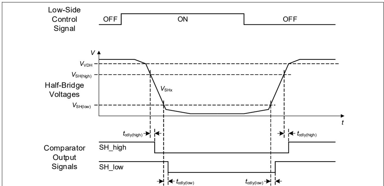
Figure 45 Timing measurement comparator thresholds and delays
