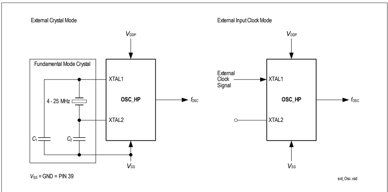
**Figure 10 TLE9868QXB20 External Circuitry for the OSC\_HP**
