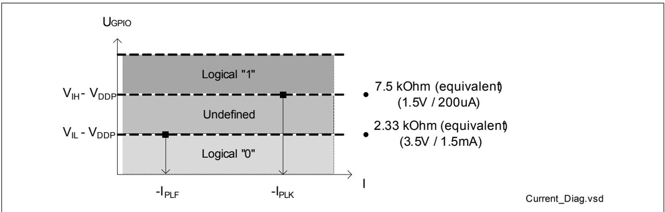
Figure 34 Pull-Up Keep and Forced Current
