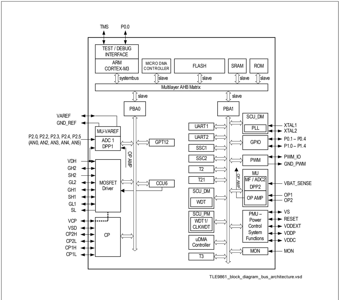
Figure 1 Block Diagram
