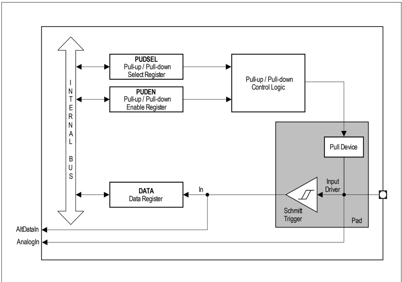
**Figure 18** General Structure of Input Port (P2)
