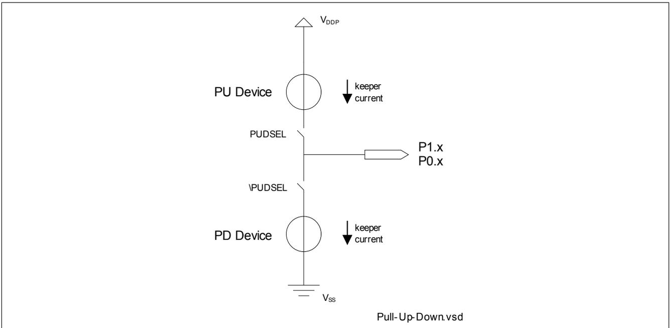
Figure 33 Pull-Up/Down Device
