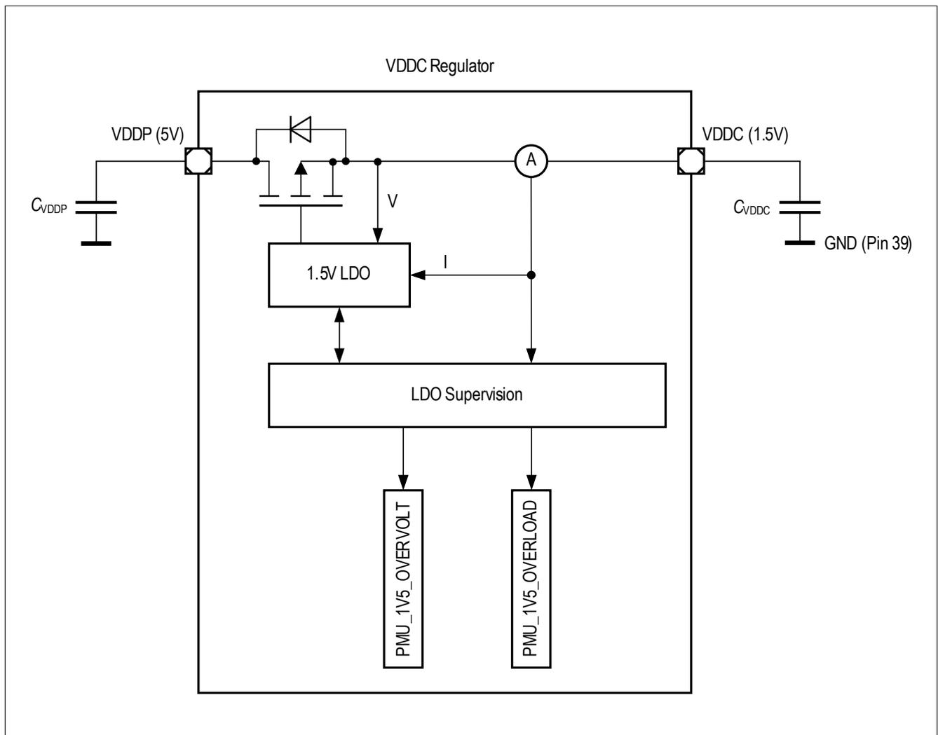
Figure 6 Module Block Diagram of VDDC Voltage Regulator
