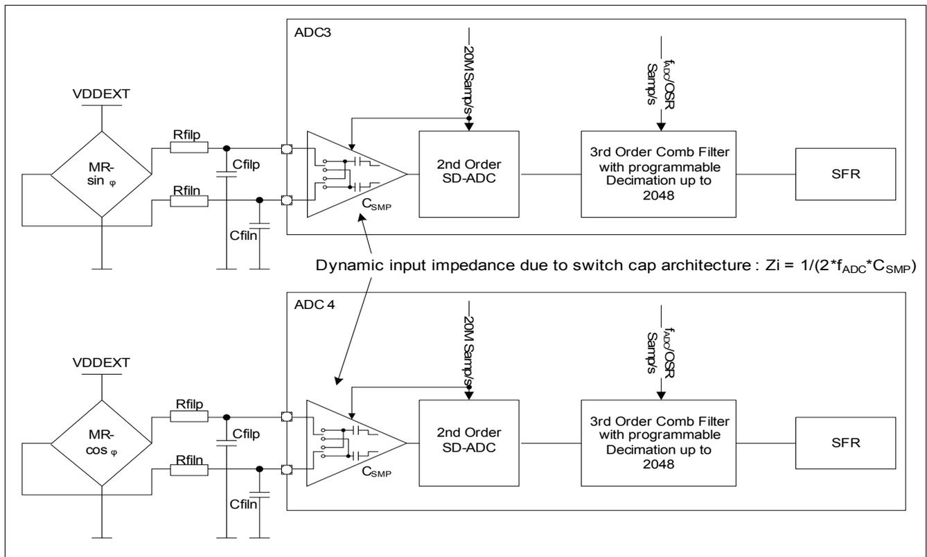
Figure 27 Application of Integrated Sigma Delta ADCs
