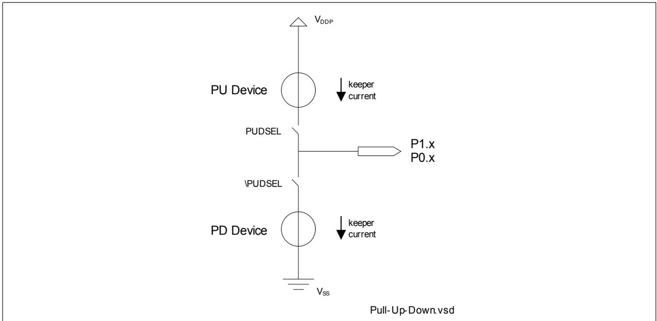
Figure 33 Pull-Up/Down Device
