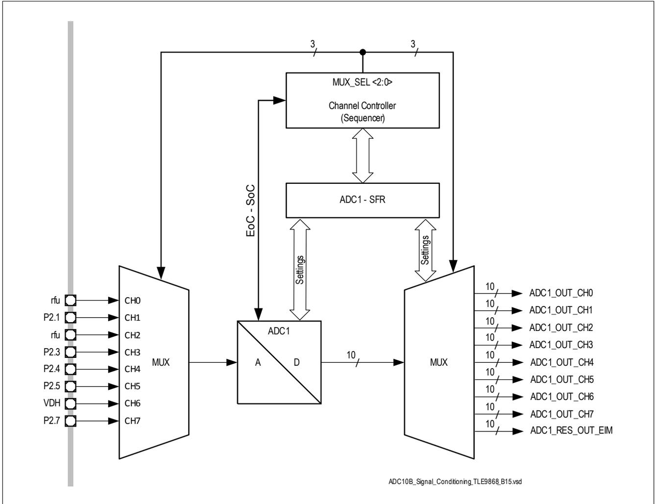
**Figure 26 ADC1 Top Level Block Diagram**
