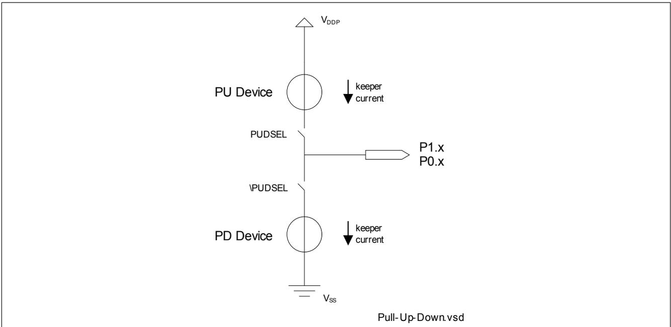
Figure 33 Pull-Up/Down Device
