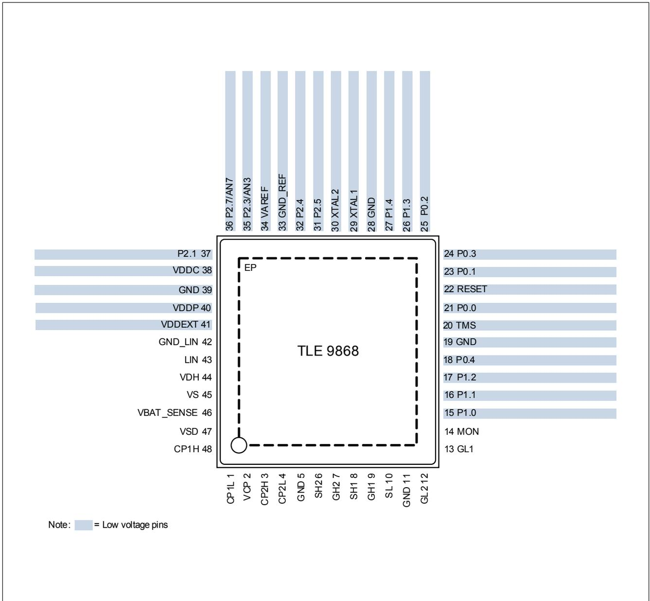
Figure 2 TLE9868QXB20 Device Pinout, VQFN-48-31 Package (top view)
