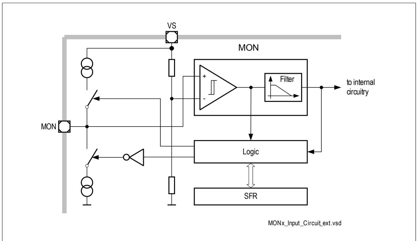
Figure 28 Monitoring Input Block Diagram
