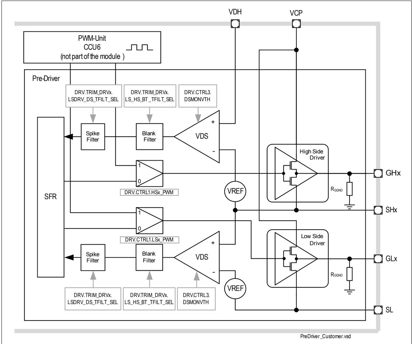
Figure 30 Driver Module Block Diagram (incl. system connections)
