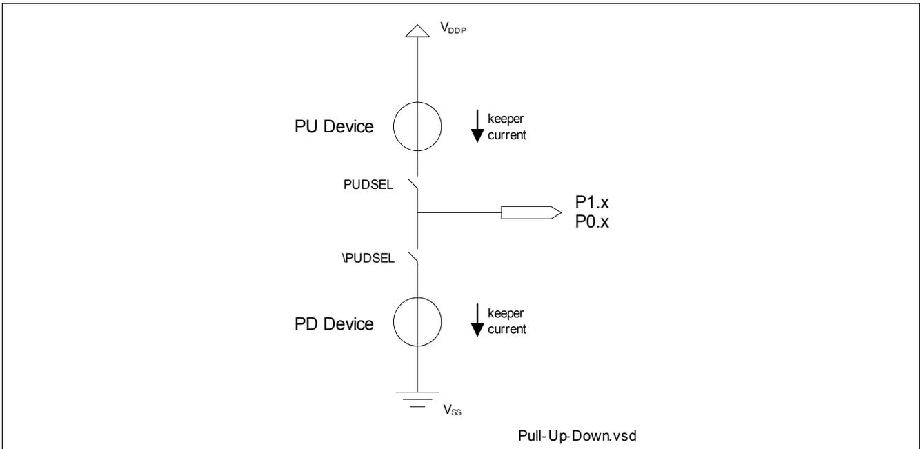
Figure 33 Pull-Up/Down Device
