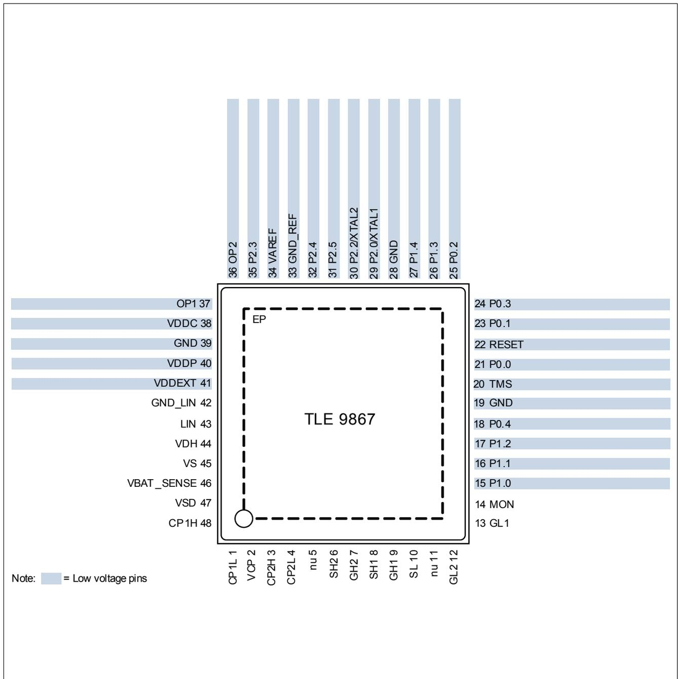
Figure 2 Device Pinout
