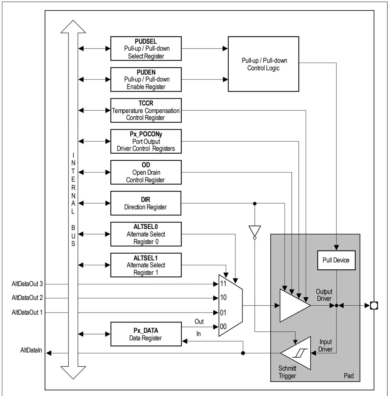
Figure 16 General Structure of Bidirectional Port (P0, P1)
