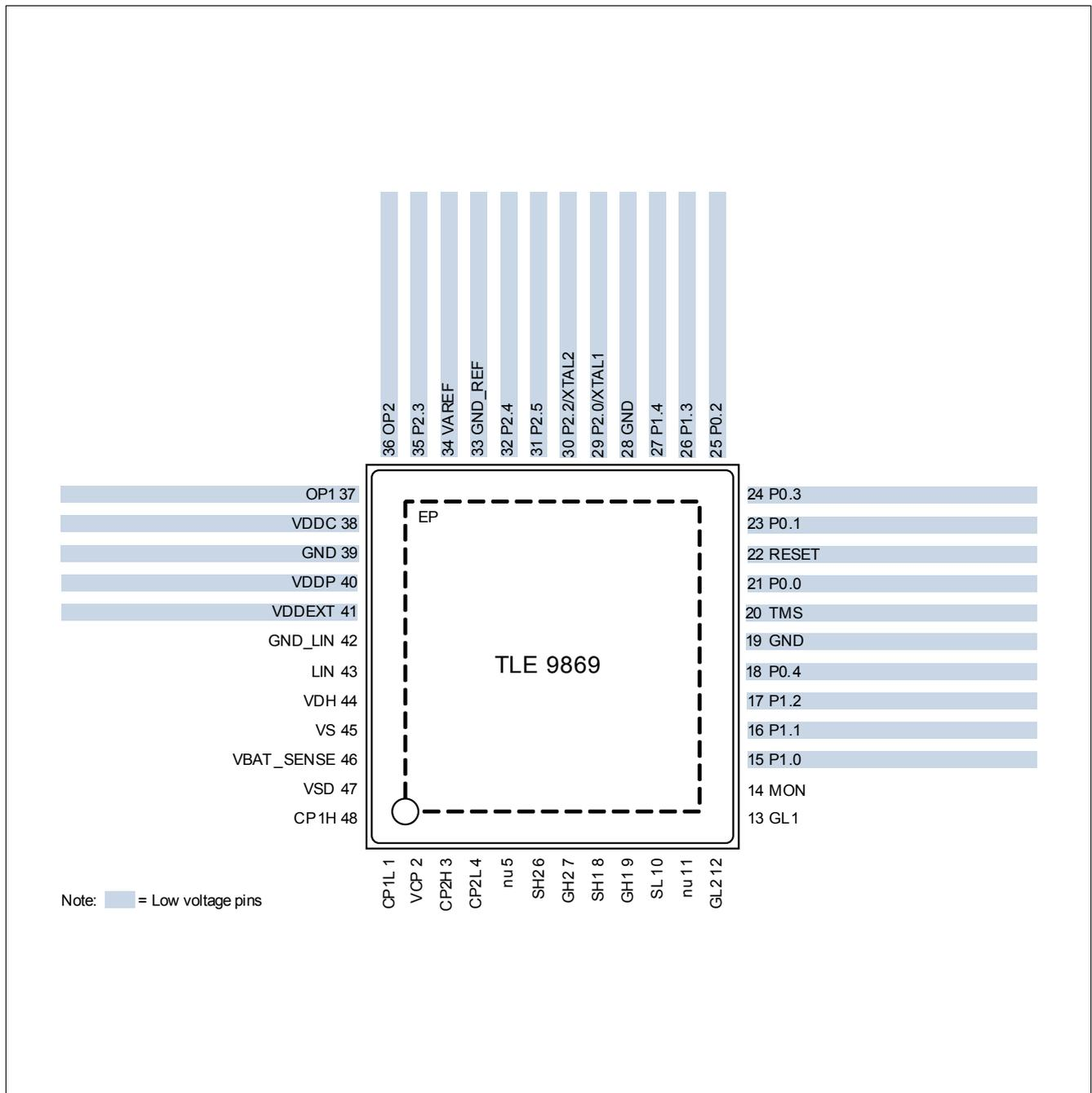
Figure 2 Device Pinout
