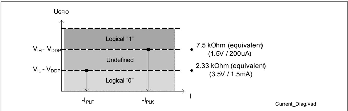
Figure 34 Pull-Up Keep and Forced Current
