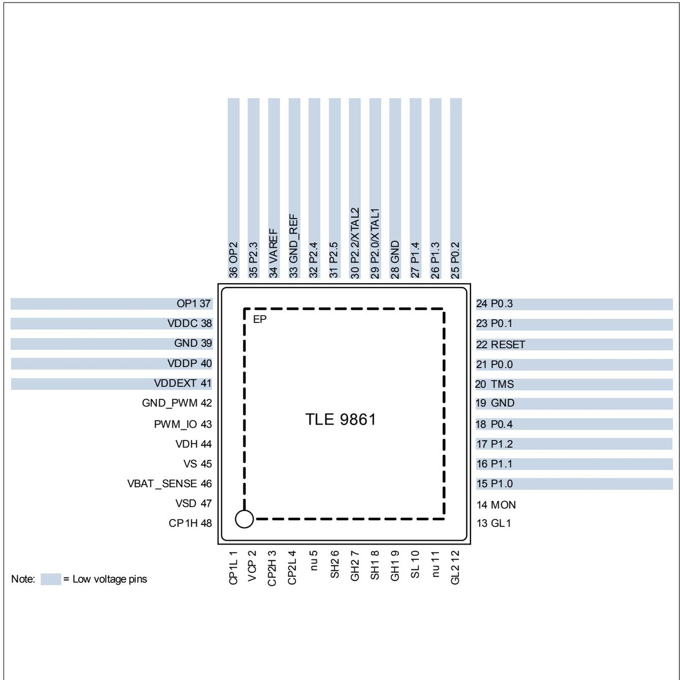
Figure 2 Device Pinout
