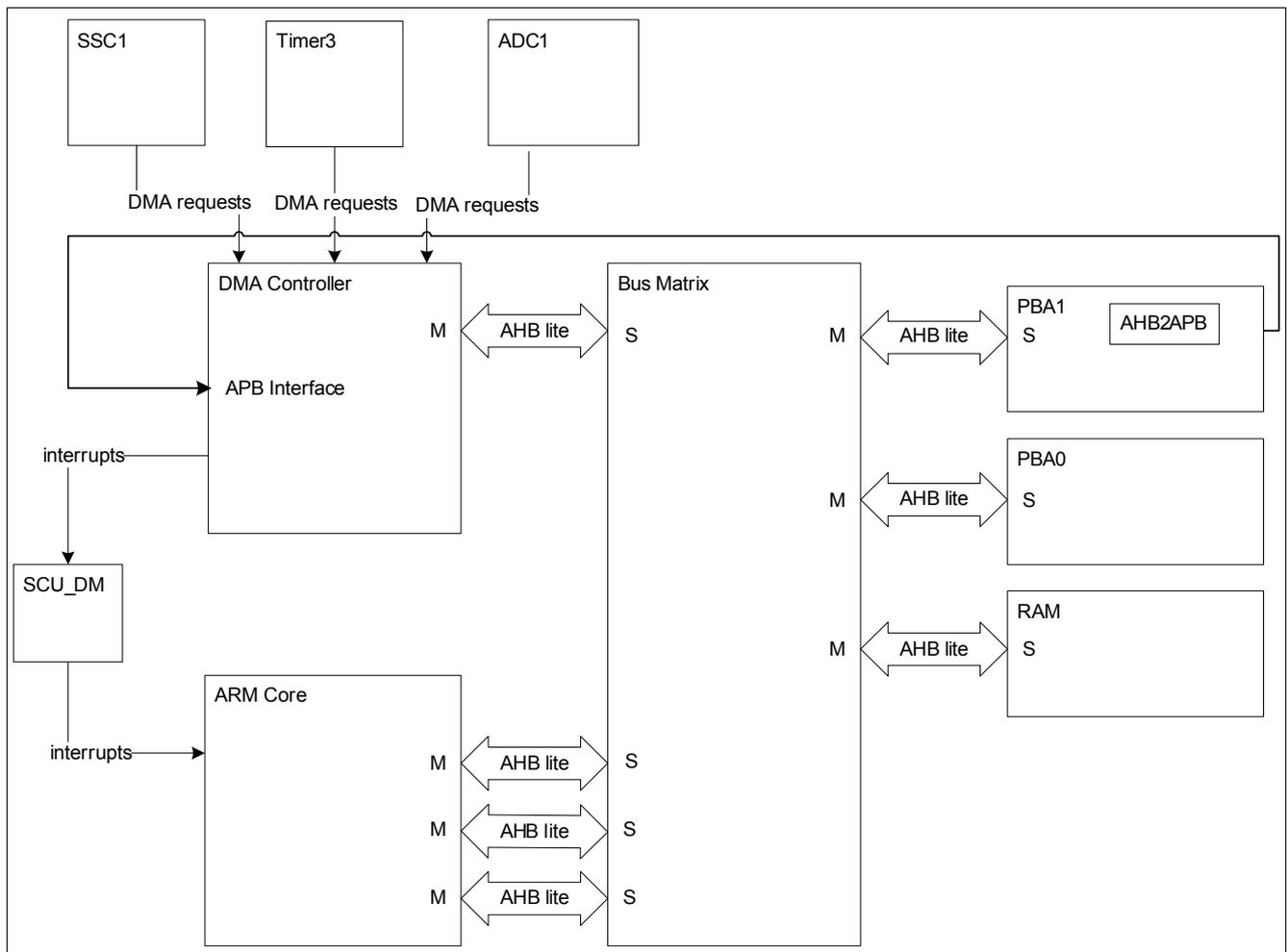
Figure 13 DMA Controller Top Level Block Diagram
