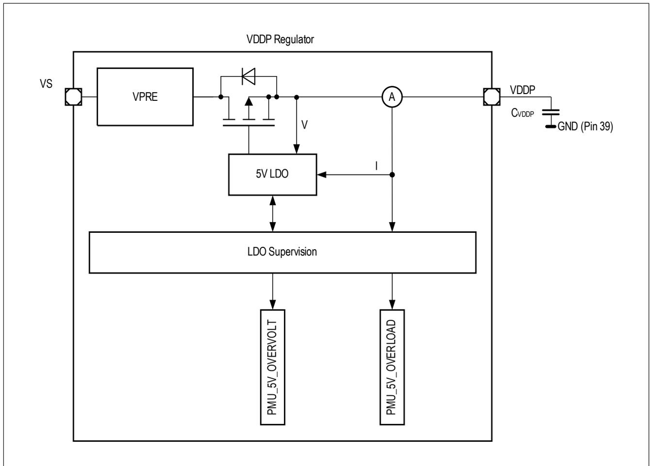
Figure 5 Module Block Diagram of VDDP Voltage Regulator
