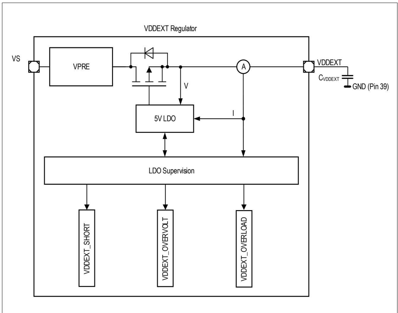
Figure 7 Module Block Diagram of External Voltage Regulator
