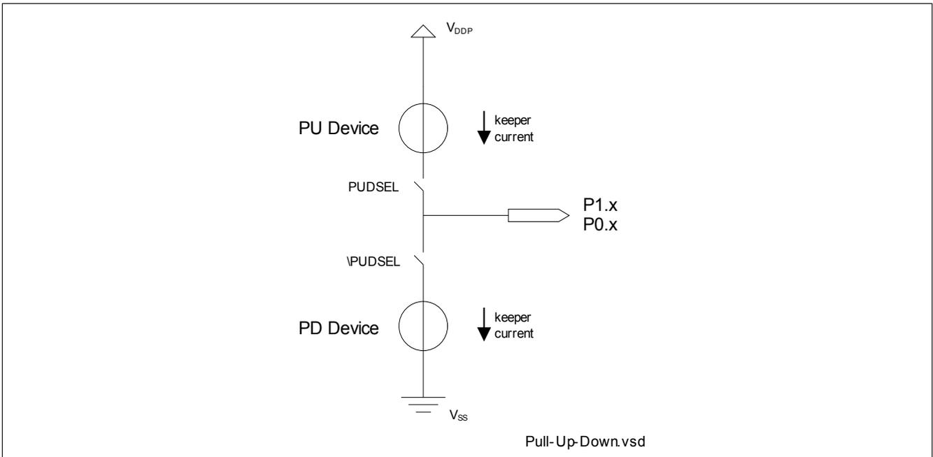
Figure 33 Pull-Up/Down Device
