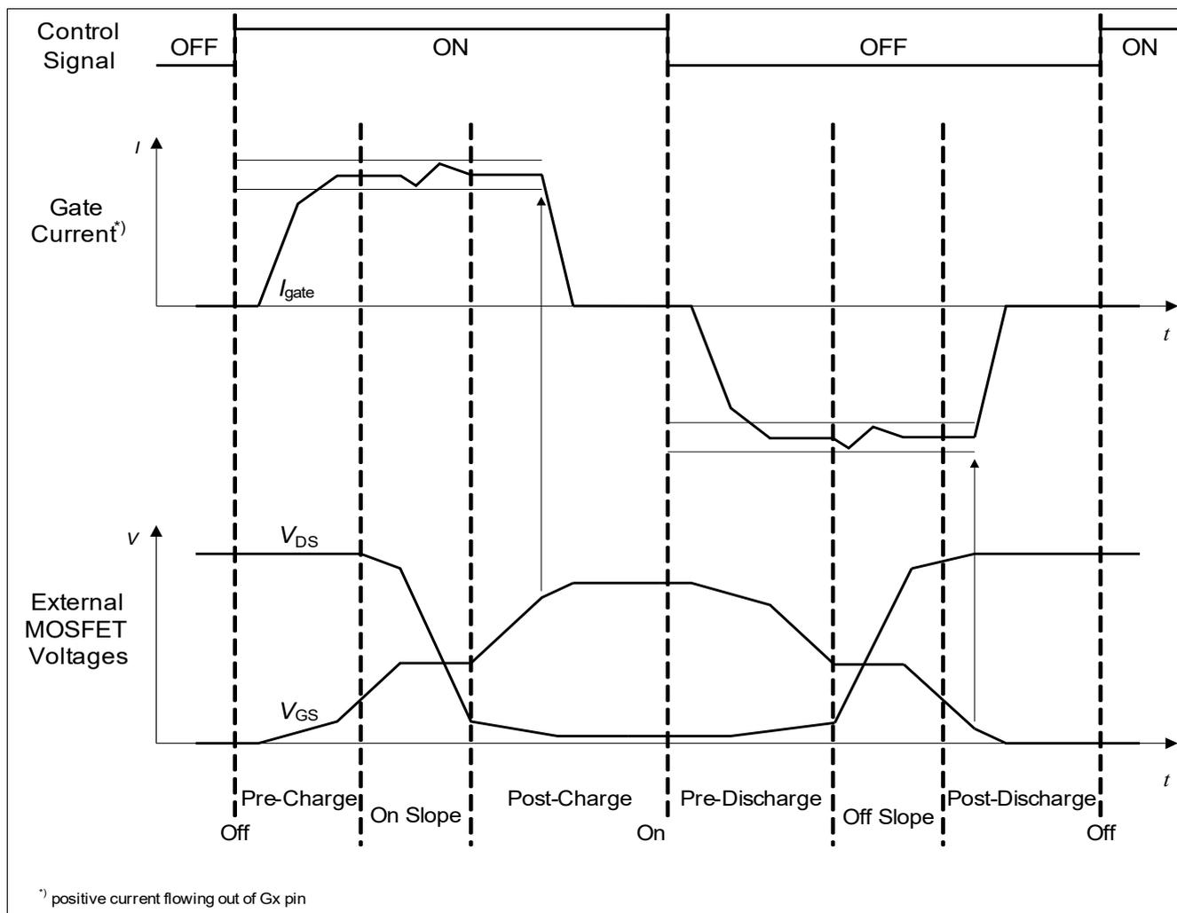
**Figure 34** Switching cycle
