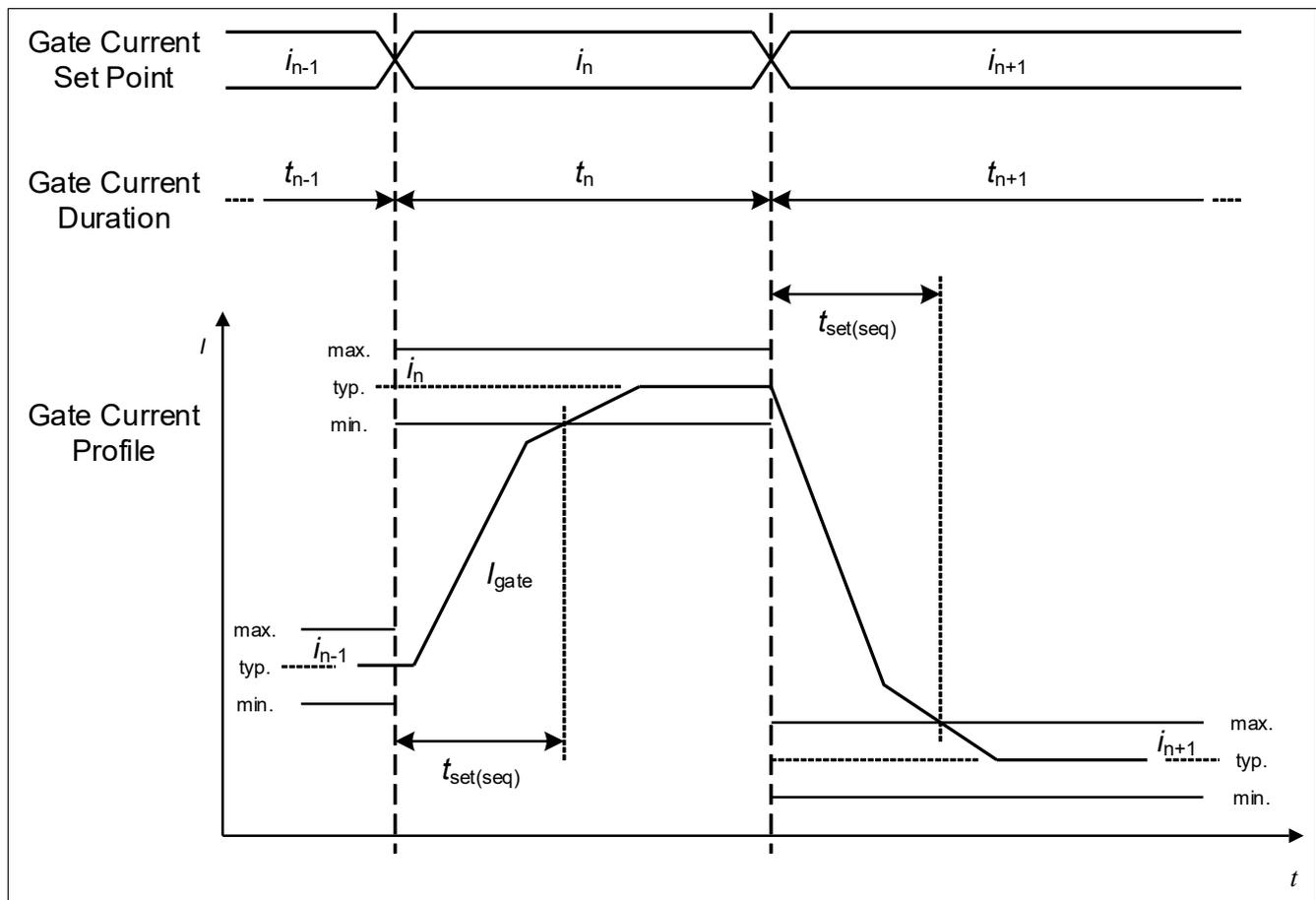
**Figure 38 Gate current settling time**
