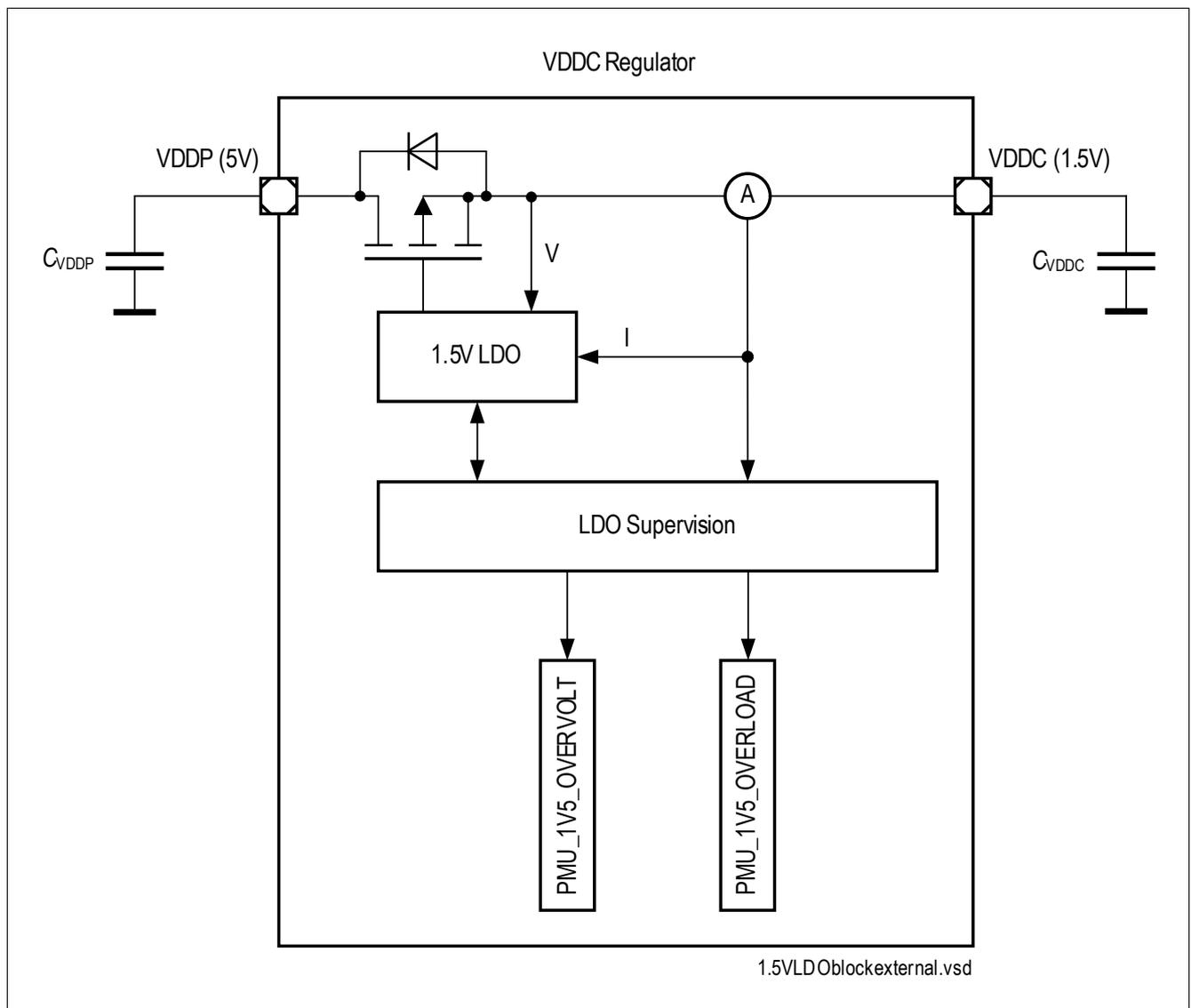
**Figure 7** Module Block Diagram of VDDC Voltage Regulator
