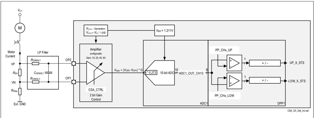
Figure 42 Simplified Application Diagram for Softshort Detection
