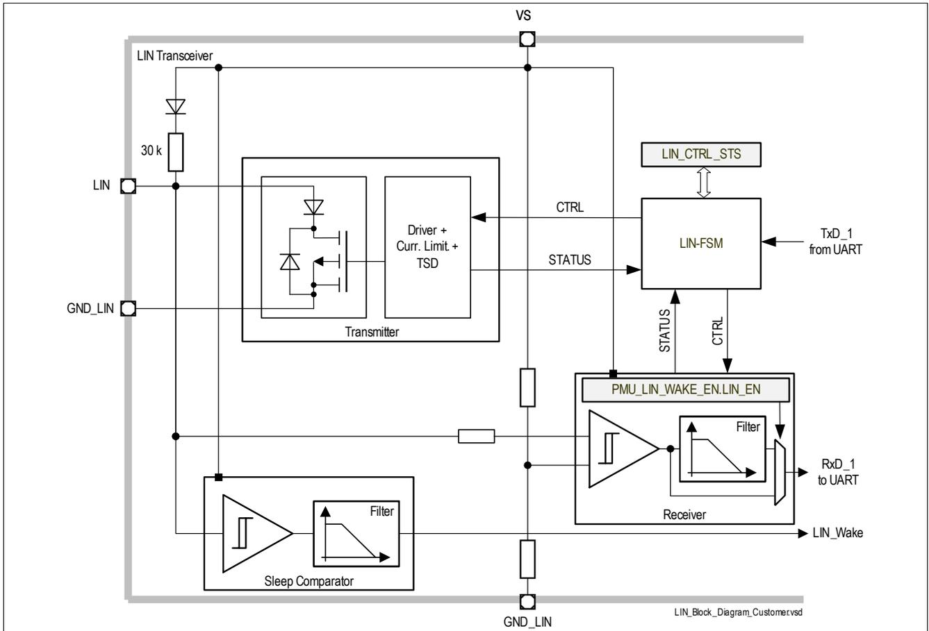
Figure 26 LIN Transceiver Block Diagram
