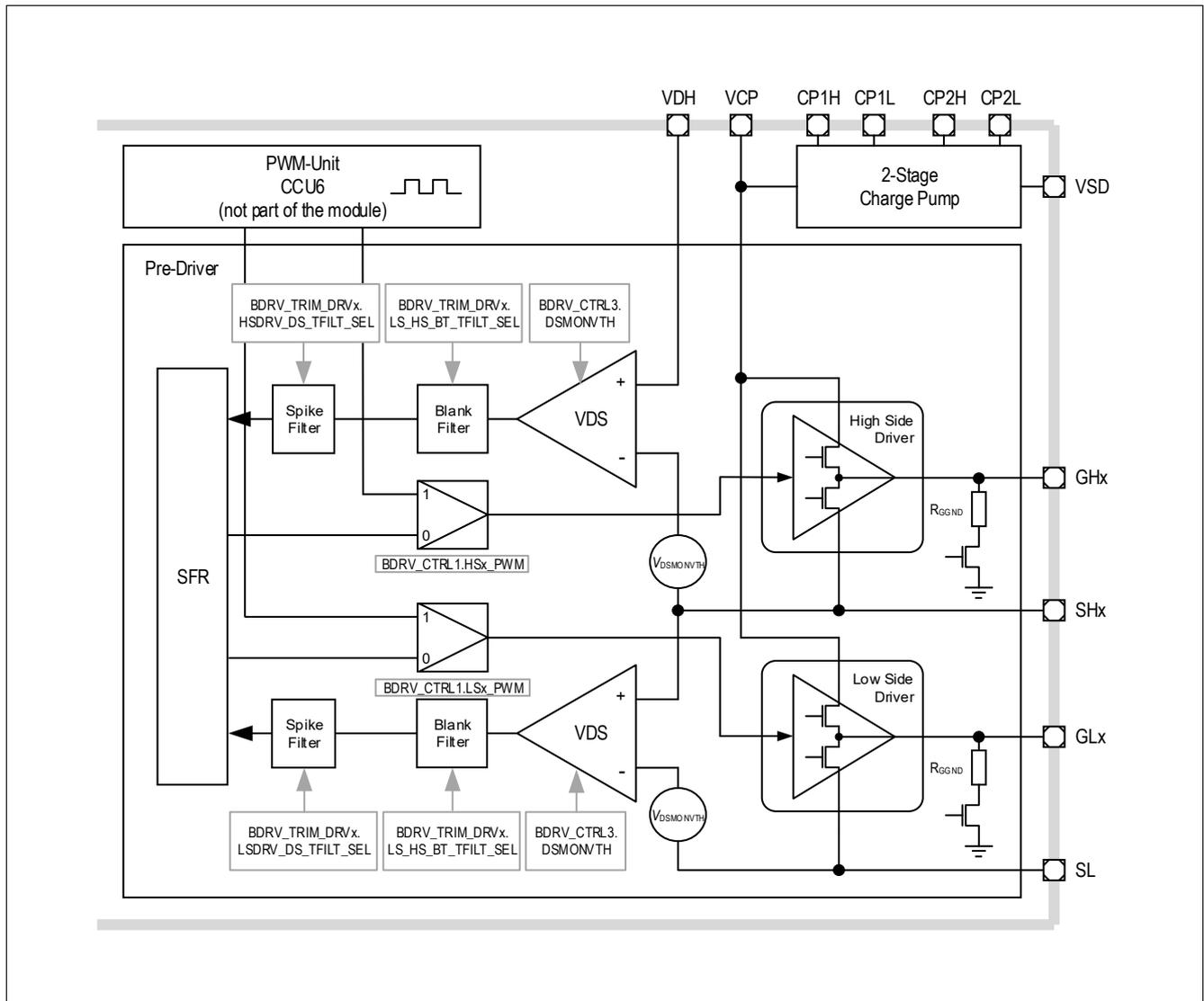
Figure 33 Driver Module Block Diagram (incl. System Connections)
