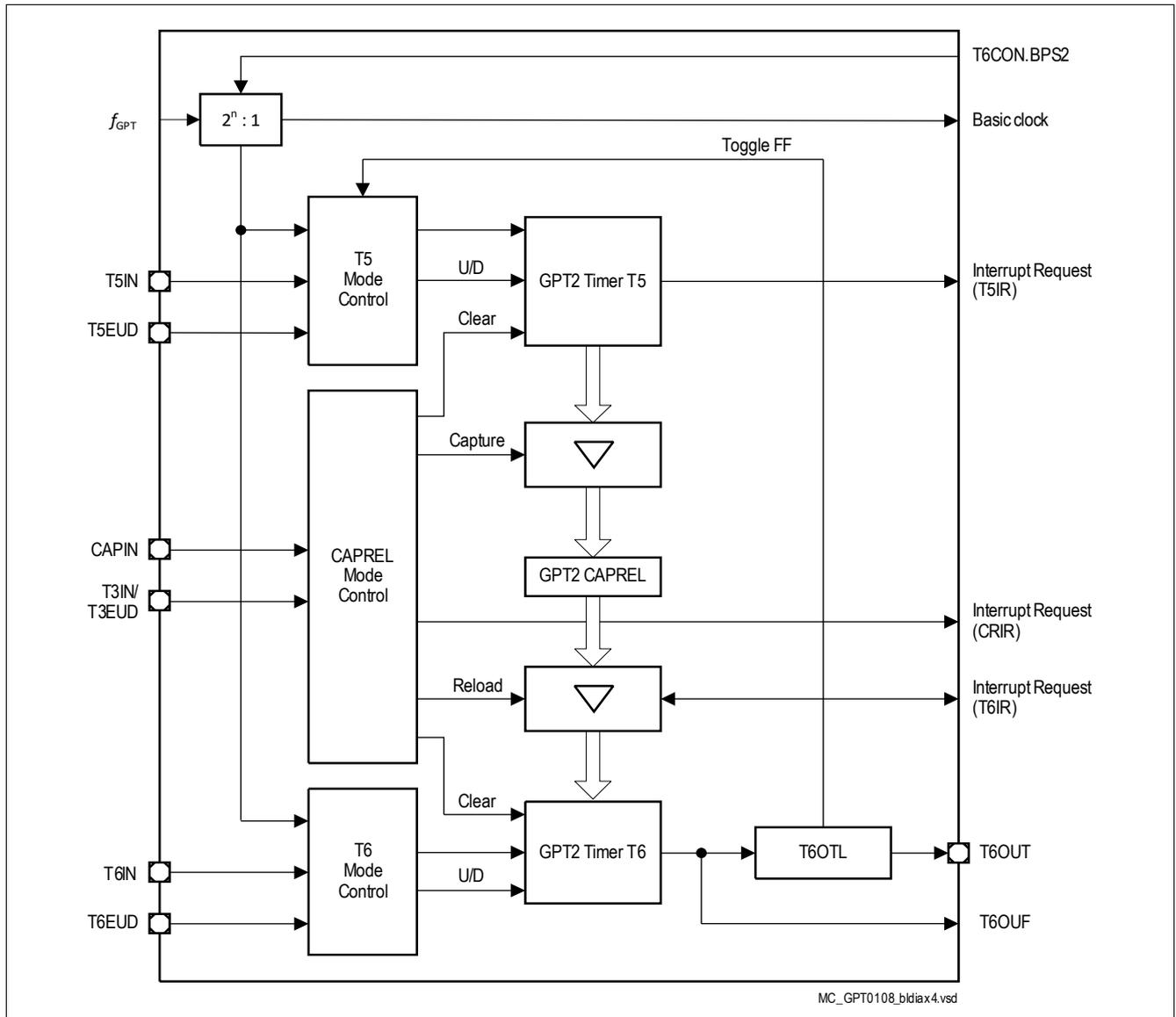
Figure 23 GPT2 Block Diagram
