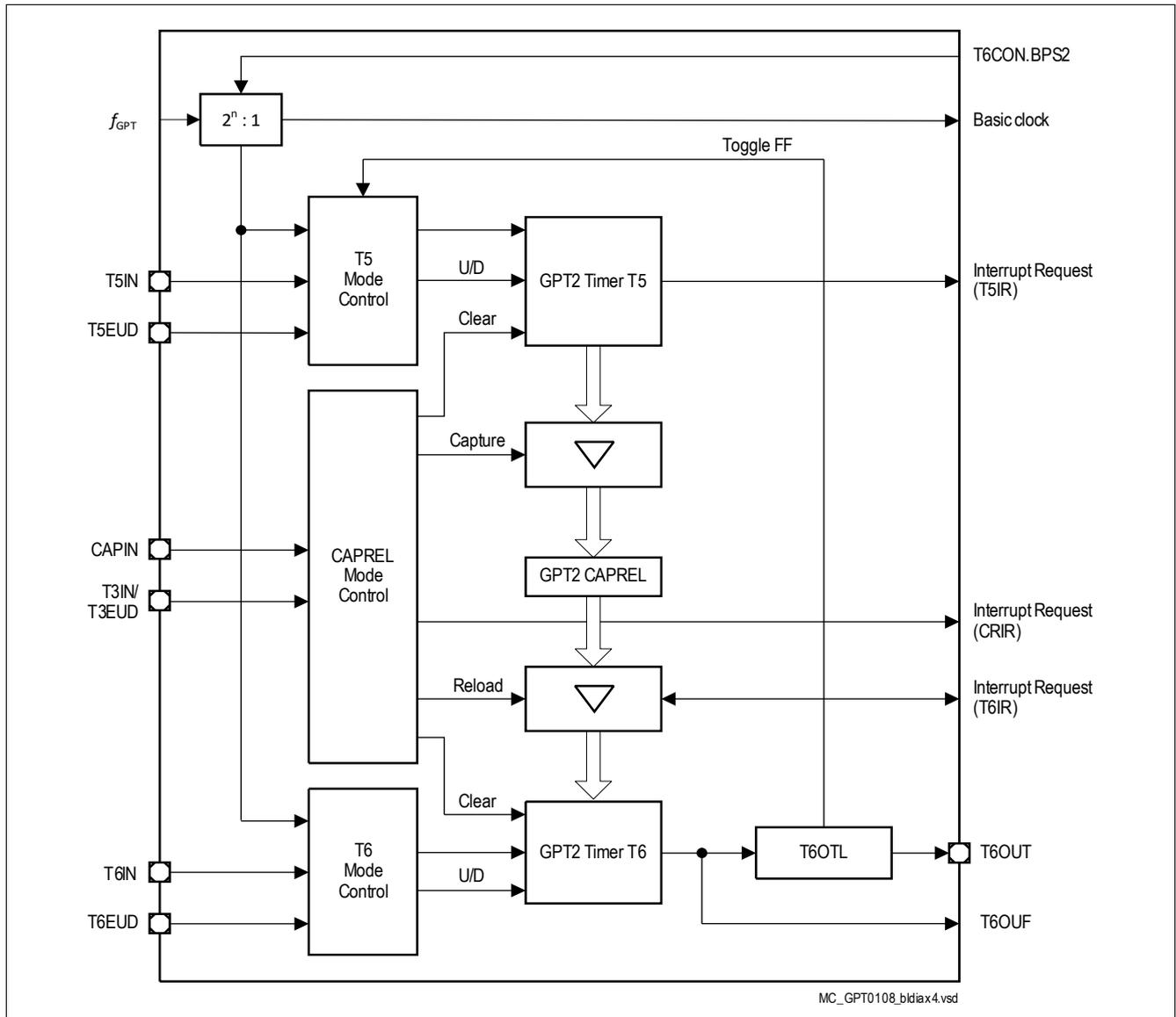
Figure 23 GPT2 Block Diagram
