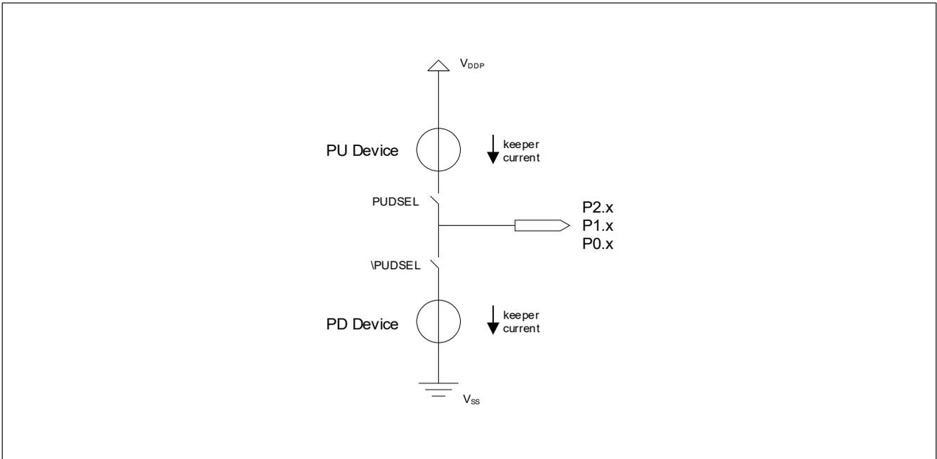
Figure 45 Pull-Up/Down Device
