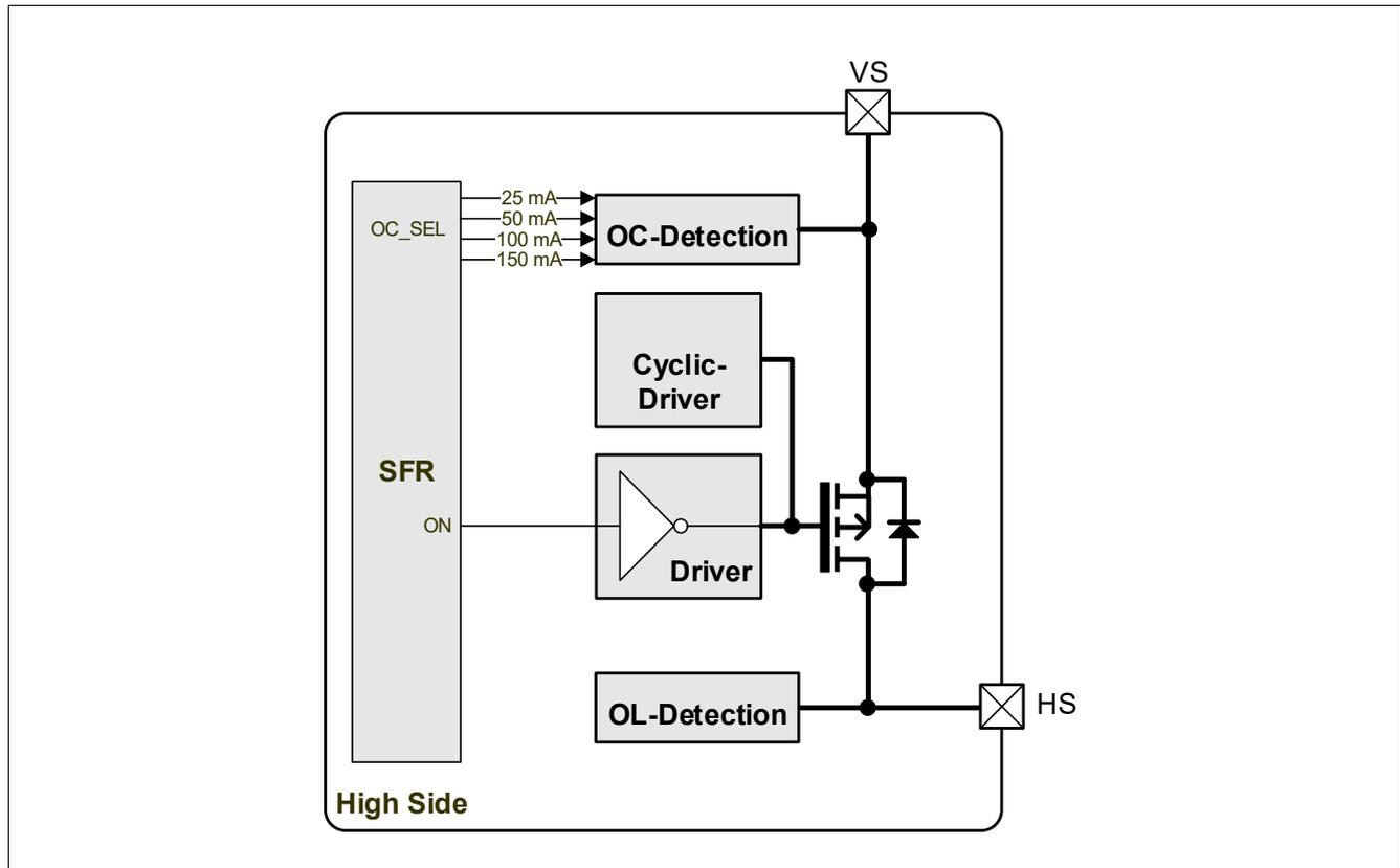
Figure 32 High-Side Module Block Diagram (incl. subblocks)
