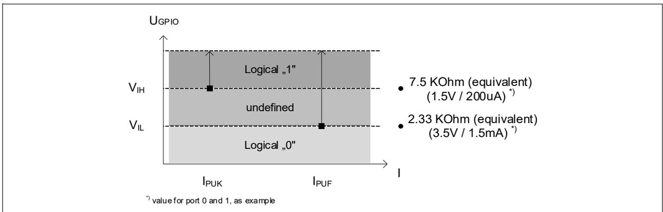
Figure 46 Pull-Up Keep and Forced Current
