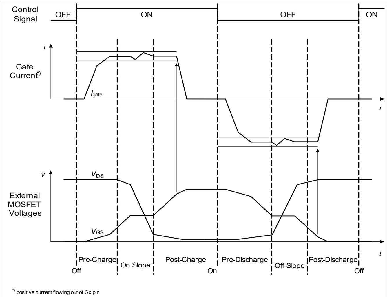
**Figure 34** Switching cycle
