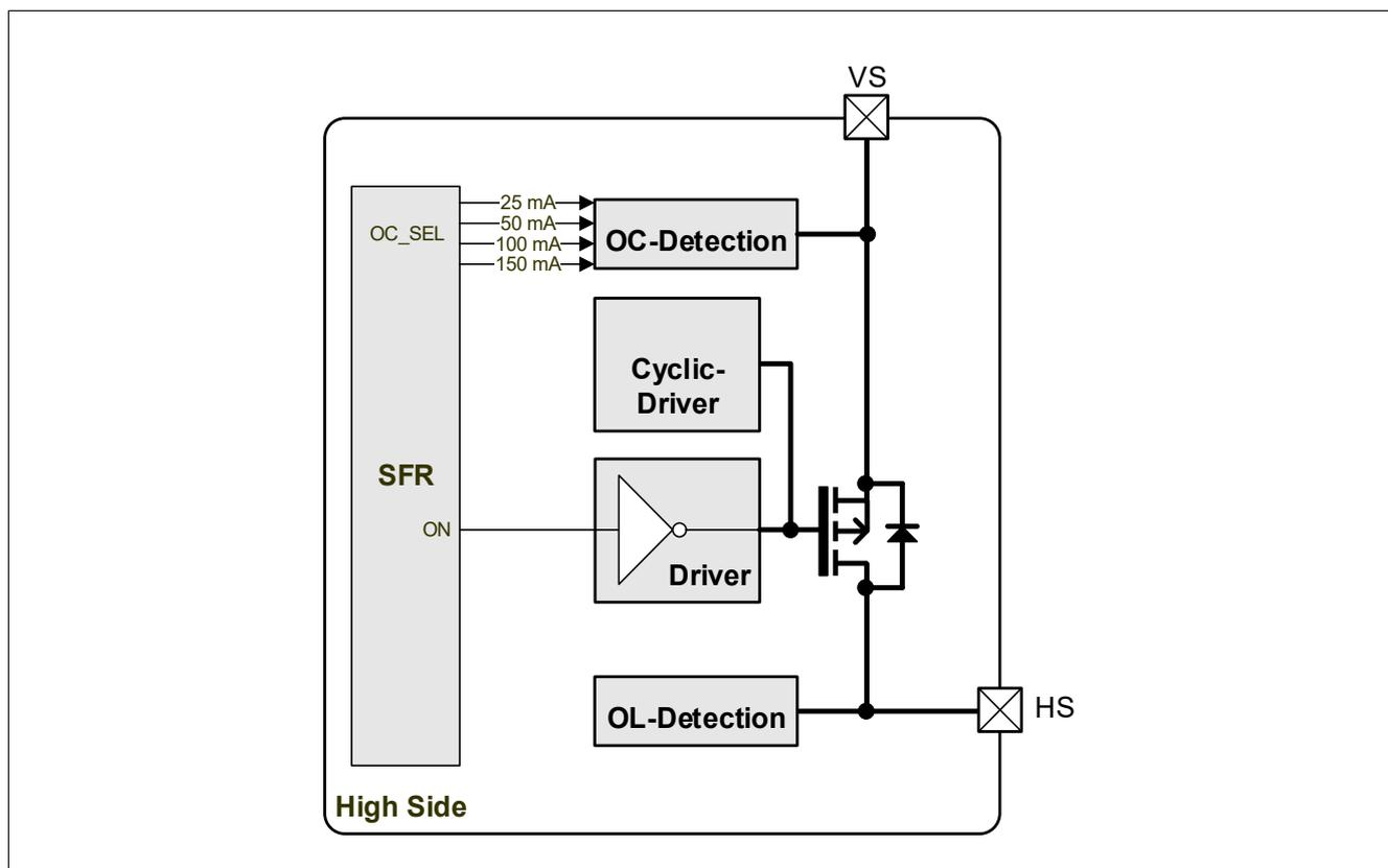
Figure 32 High-Side Module Block Diagram (incl. subblocks)
