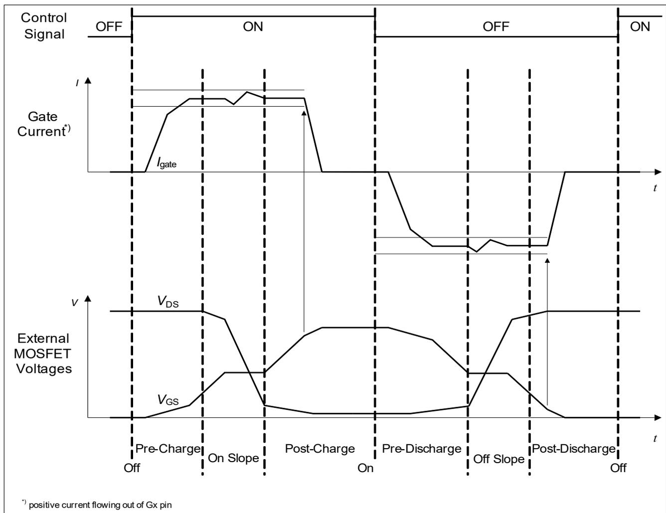
**Figure 34** Switching cycle
