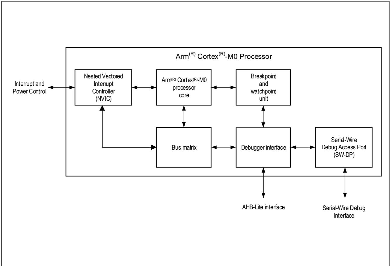
Figure 15 Arm® Cortex®-M0 Block Diagram
