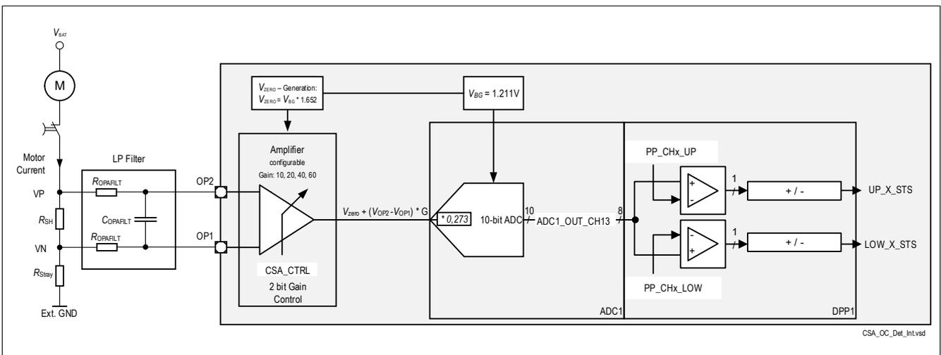
Figure 42 Simplified Application Diagram for Softshort Detection
