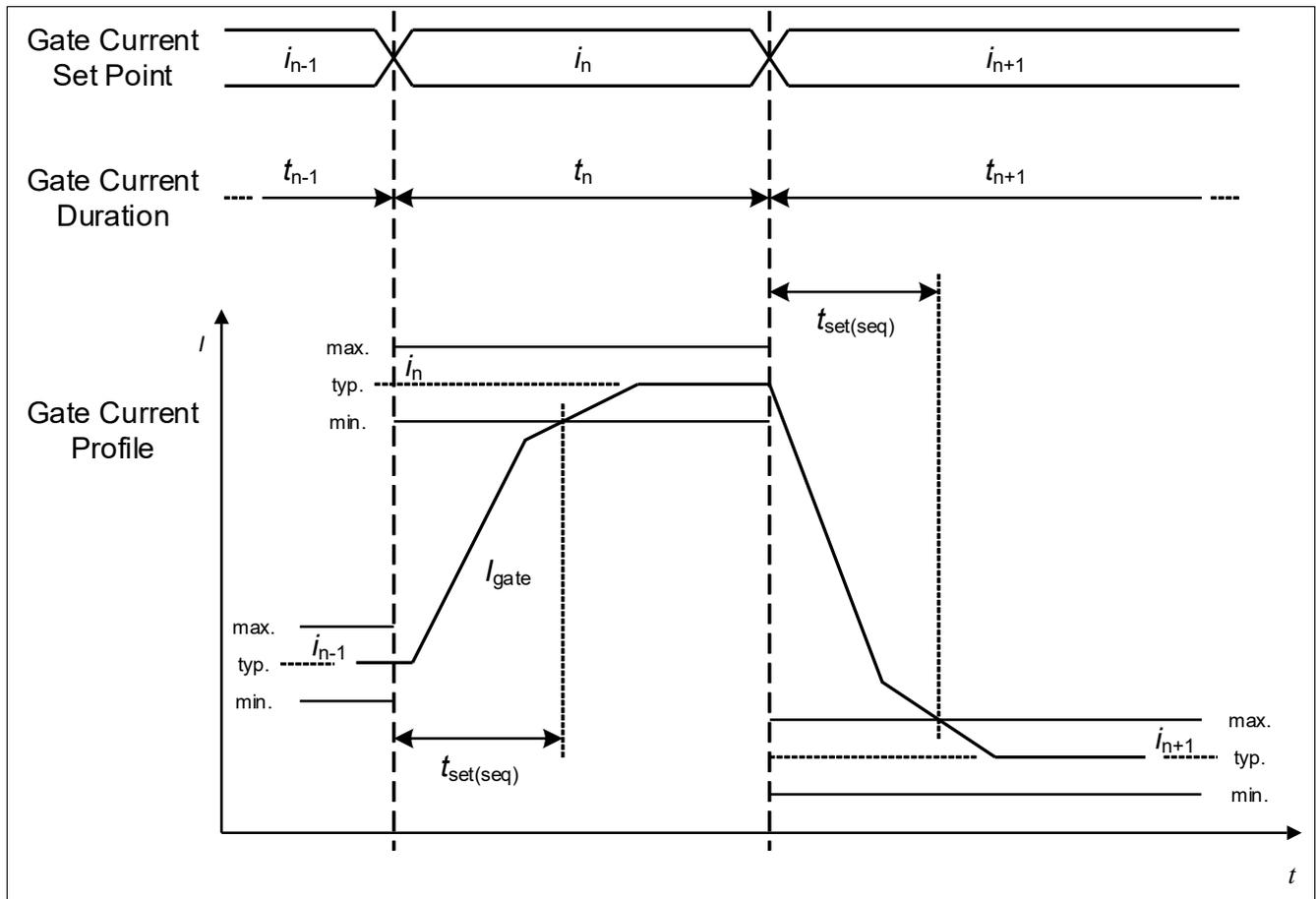
Figure 38 Gate current settling time
