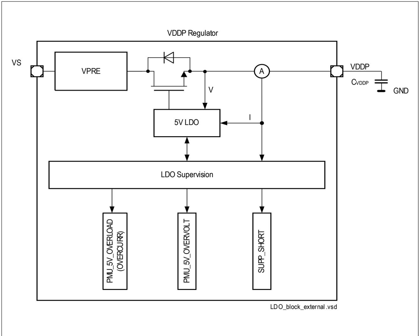
Figure 6 Module Block Diagram of VDDP Voltage Regulator
