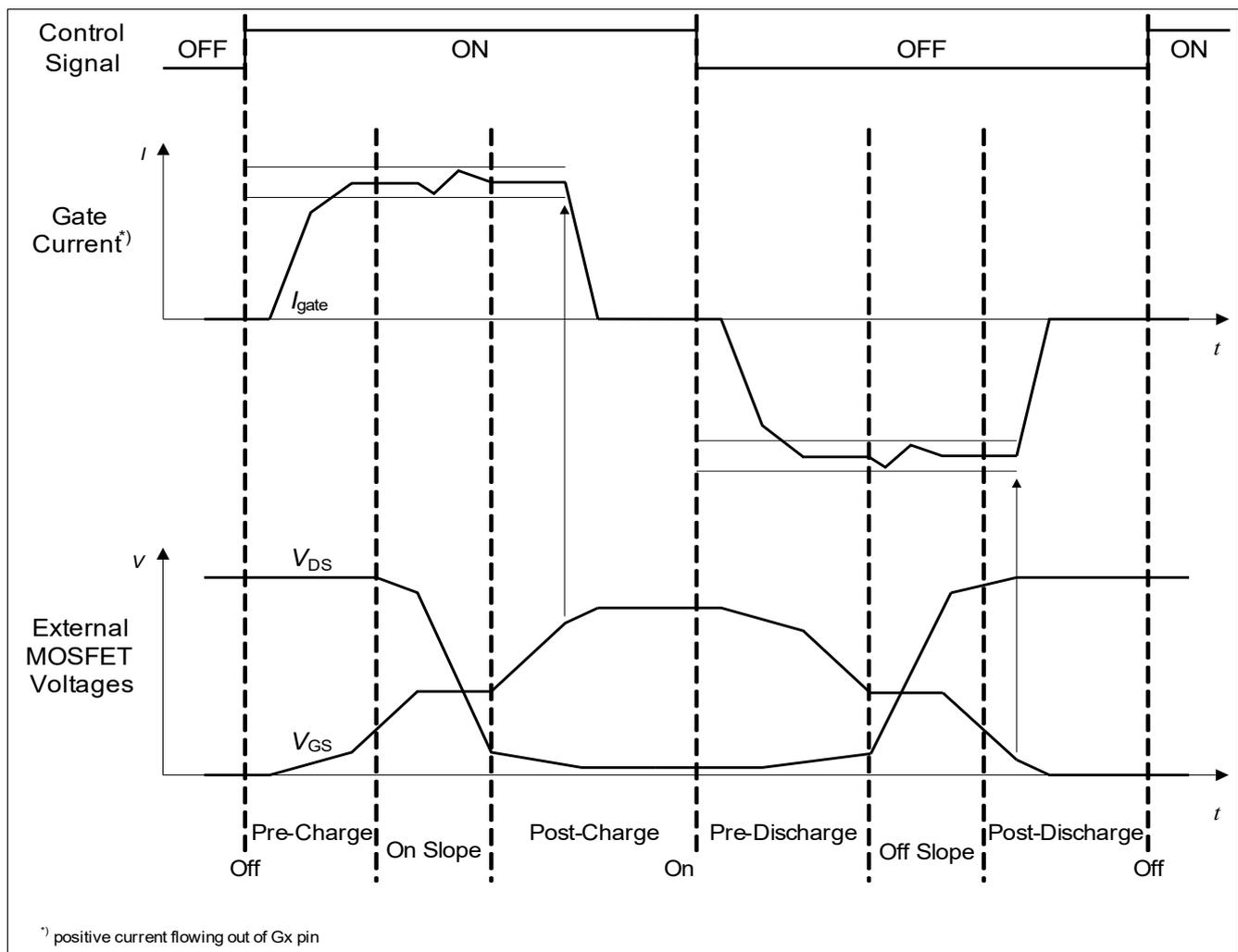
**Figure 34** Switching cycle
