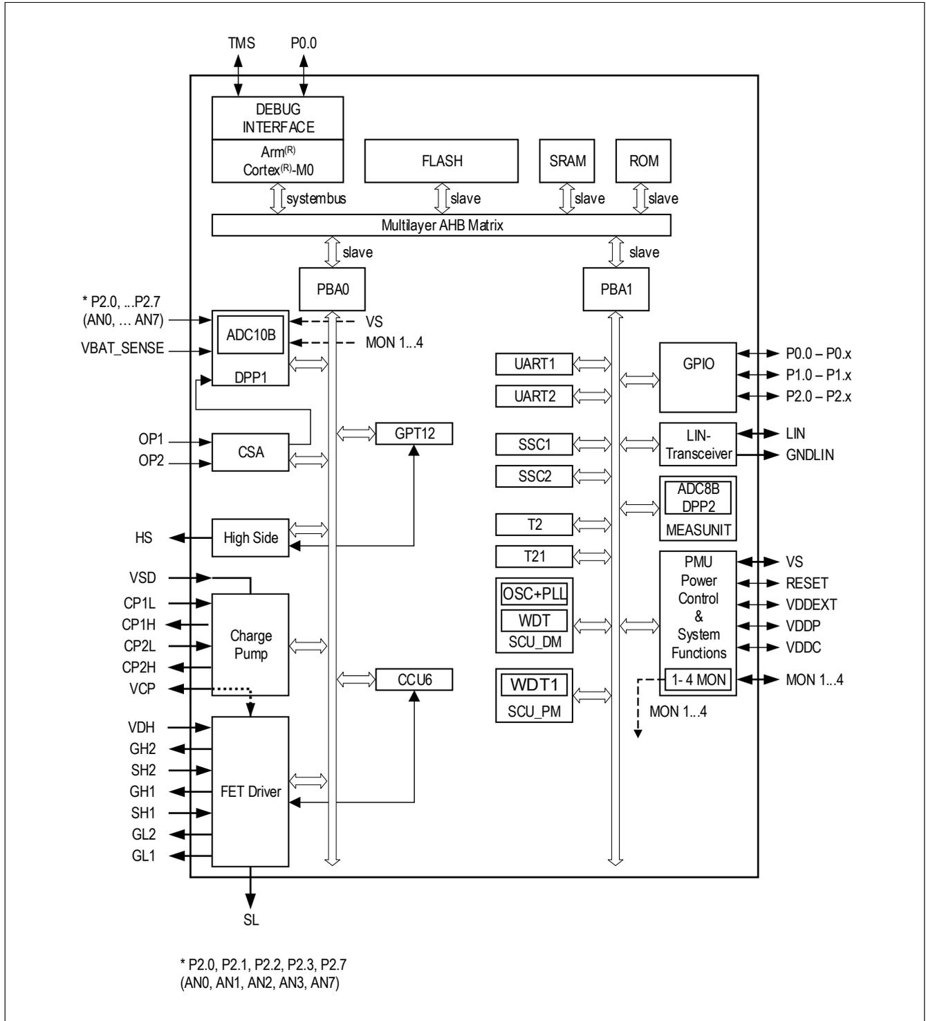
Figure 1 Block Diagram TLE9854QX
