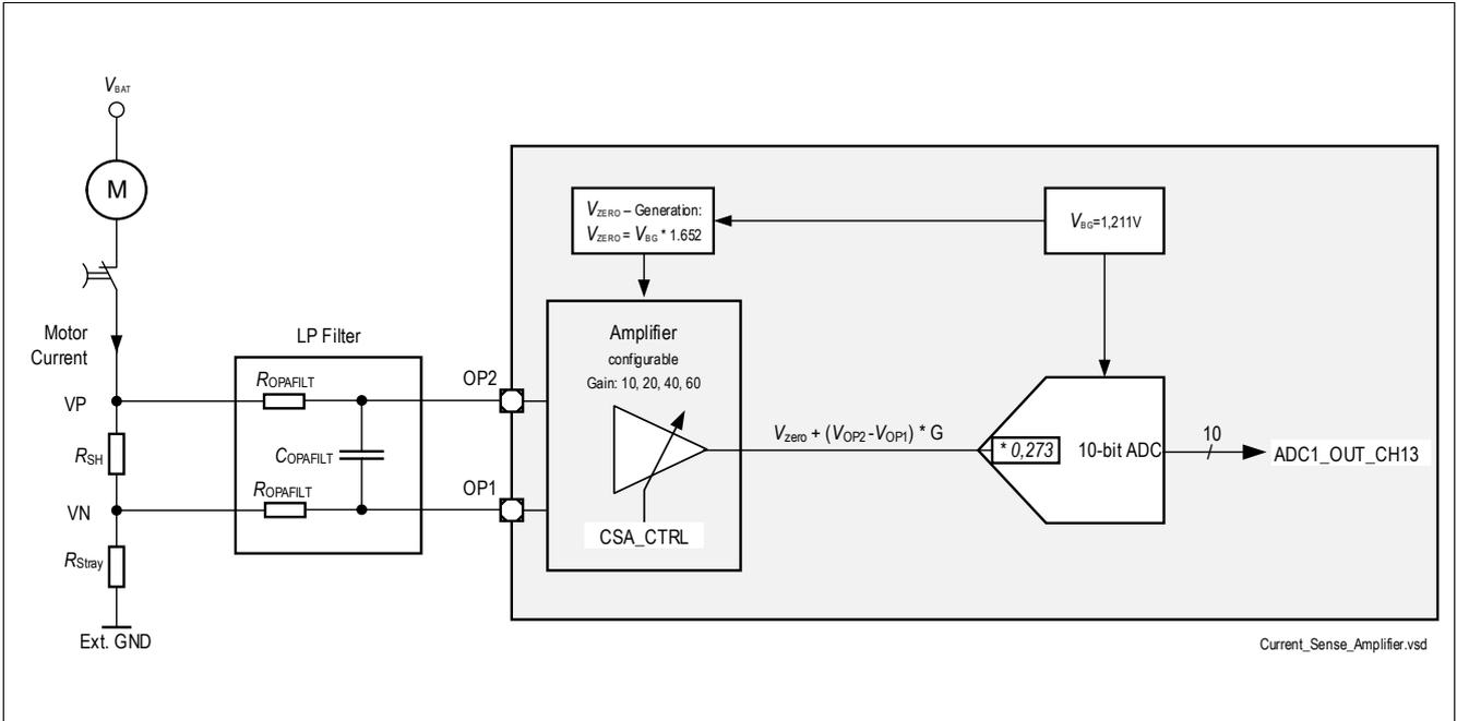
Figure 41 Simplified Application Diagram
