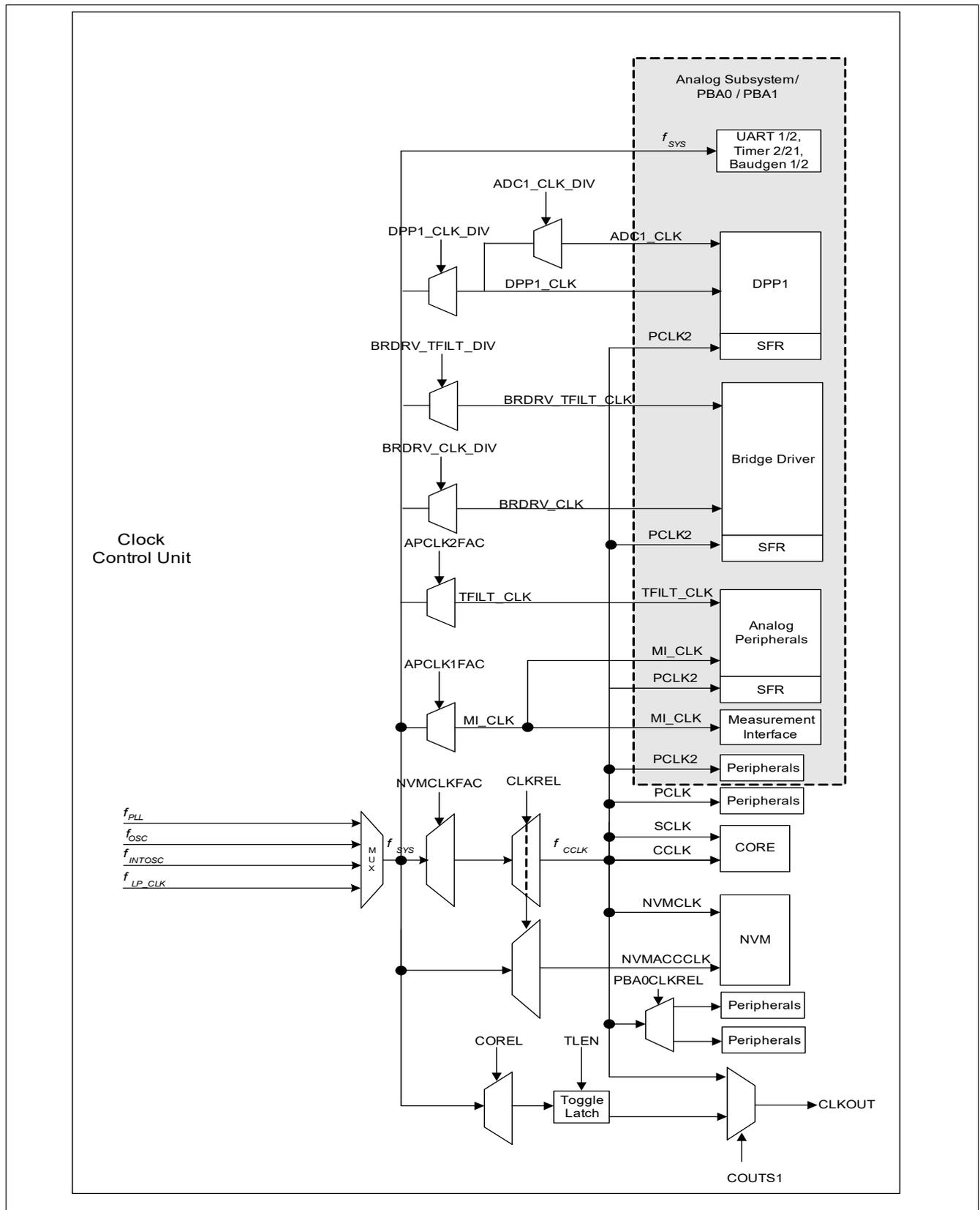
Figure 13 Clock Generation from  $f_{sys}$ ; CLKOUT Generation
