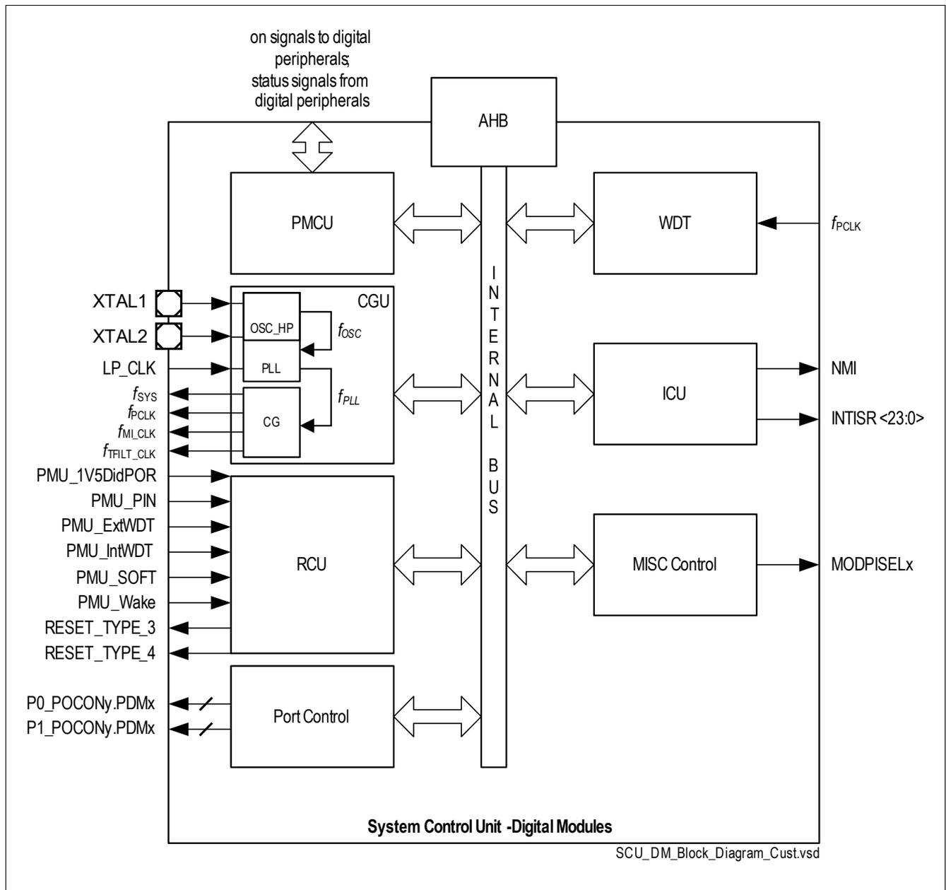
Figure 10 System Control Unit - Digital Modules Block Diagram
