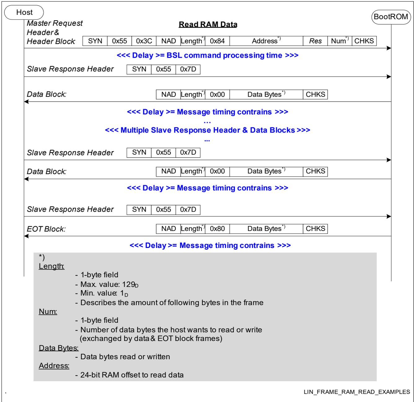
Figure 4-13 BSL RAM Read Access Frame Examples
