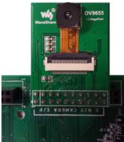
Figure 11: OV9655 camera connected to DCMI port
