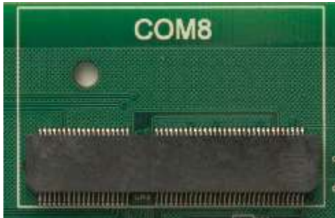
Figure 7: COM8 connector. The notch is located on the bottom-right corner of the connector.
