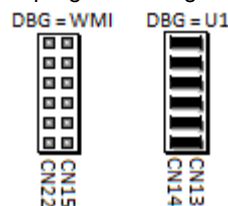
Figure 6: Jumpers between CN13 and CN14 pins – selects STM32F407IGT6/STM32F429IIT6 MCU to program/debug
