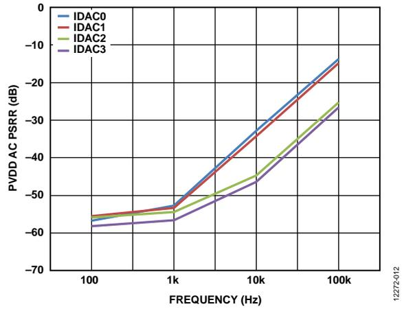
Figure 12. Typical PVDD AC PSRR vs. Frequency
