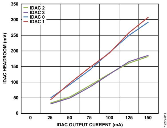
Figure 11. Typical IDAC Headroom vs. IDAC Output Current
