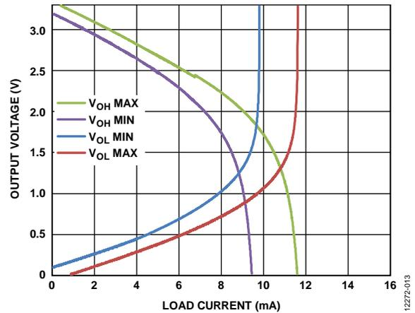
Figure 13. Typical Output Voltage vs. Load Current
