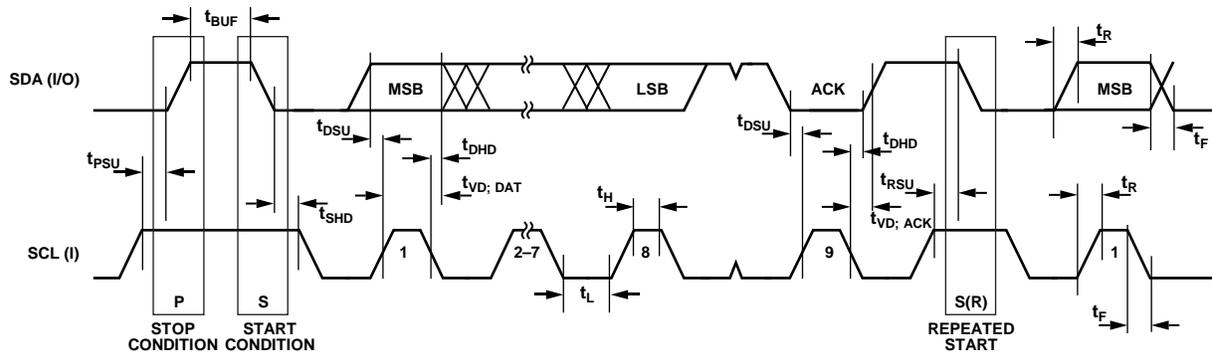
Figure 2. I<sup>2</sup>C Compatible Interface Timing
