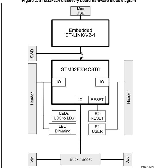
Figure 2. STM32F334 discovery board hardware block diagram
