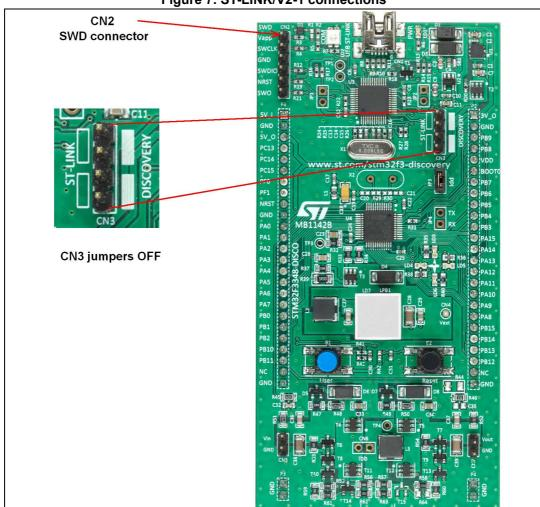
Figure 7. ST-LINK/V2-1 connections
