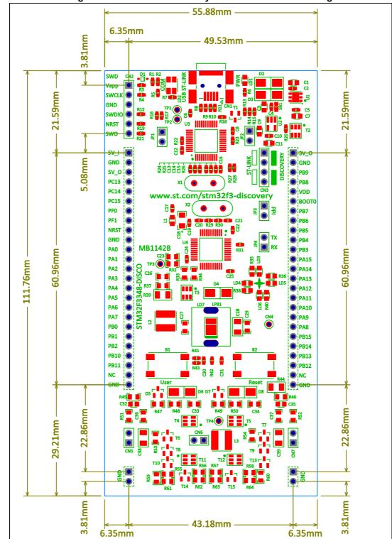
Figure 8. STM32F334 discovery board mechanical drawing
