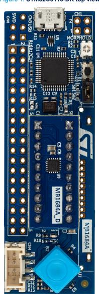
Figure 1. STM32C0116-DK top view
