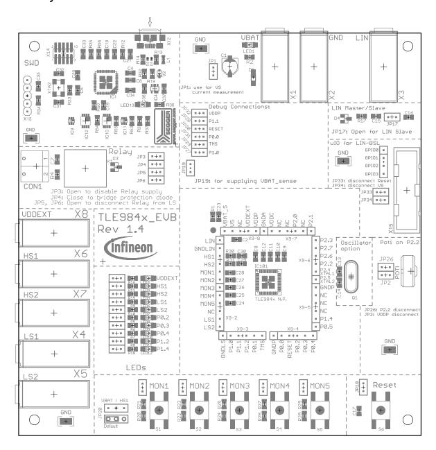
Figure 8 Parts placement
