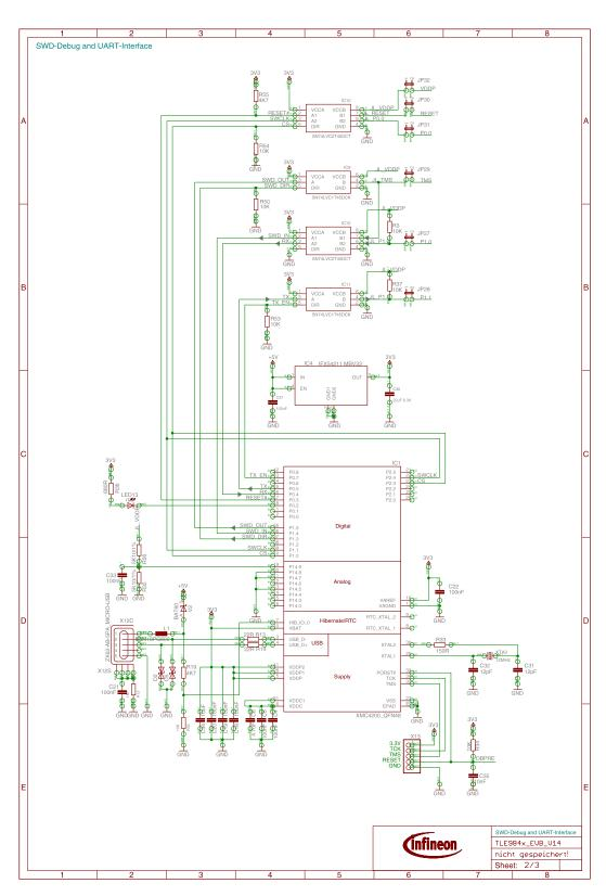
Figure 7 Onboard debug cicuit
