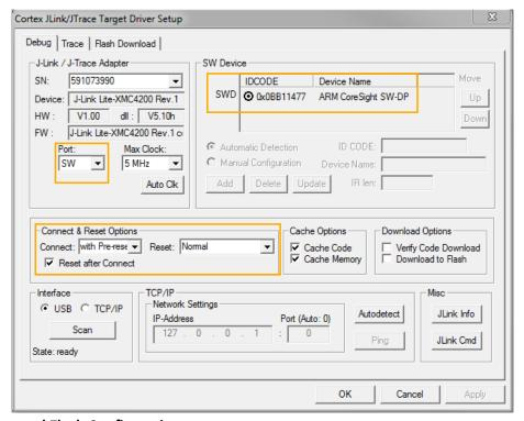
Figure 5 Debug and Flash Configuration
